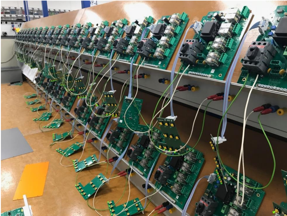
Figure 15: Hotraco Agri circuit boards in production at their manufacturing facility. (Photo: author's own)
