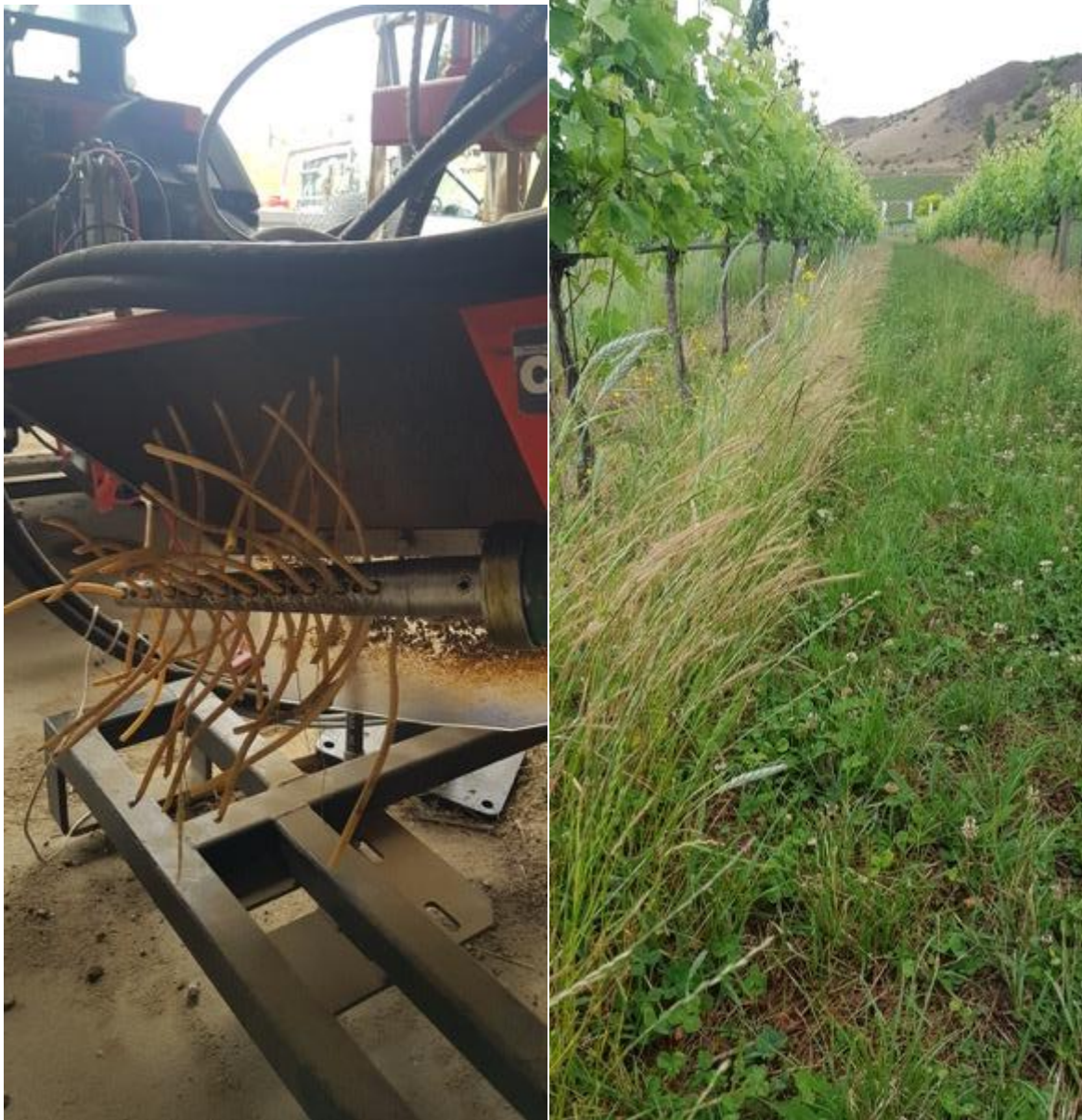
Left - Figure 17. New over-row cord weeding machine. Terra Sancta Vineyard, Central Otago. (Author, 2019)
