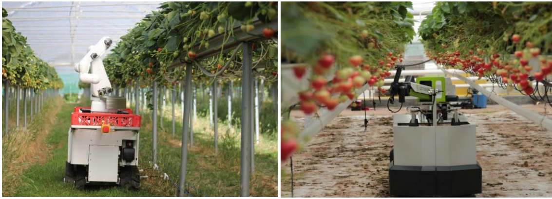
Figure 34. Robots from Dogtooth and Octinion respectively designed to pick soft fruit.
