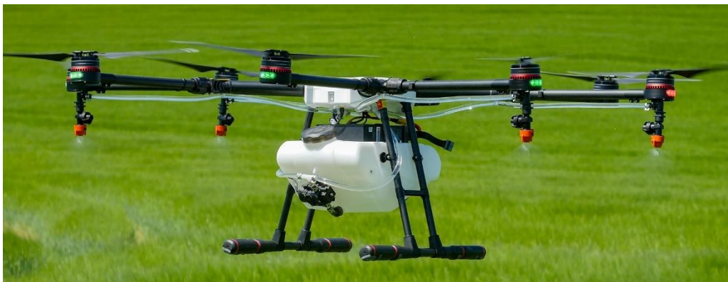
Figure 10: A DJI Agras Mg1 multirotor UAS flying over a crop while spraying (water). Image source "Drone Ag".
