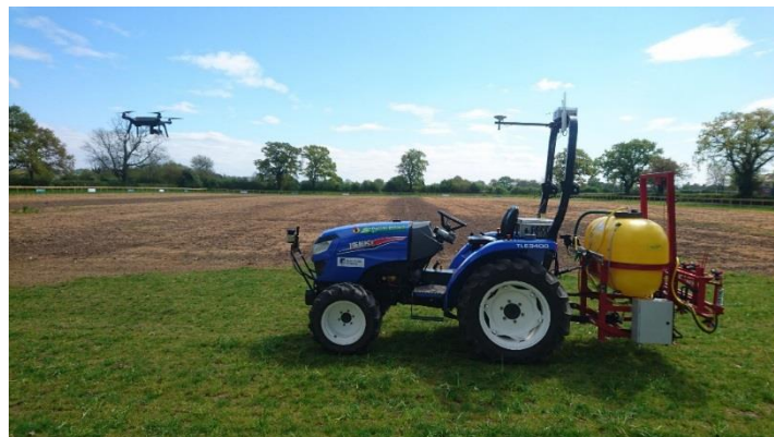
Figure 2: Automated machines growing the first arable crop remotely, without operators in the driving seats or agronomists on the ground.” Photos author's own from Hands Free Hectare project
