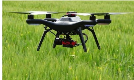
Figure 9: 3DR Solo drone adapted to hold a Multispectral camera. Author's own.
