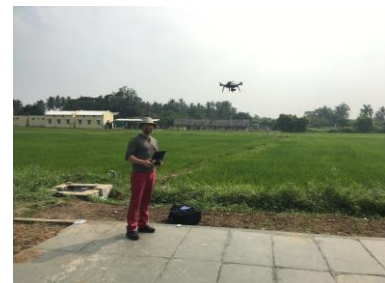
Figure 13 : The author flying a UAS mapping a rice crop with a multispectral camera. Author's own.
