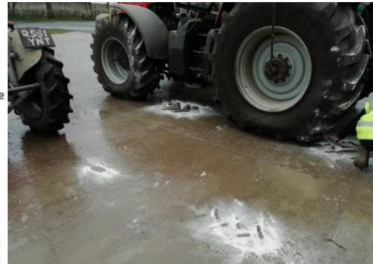
Figure 4: shows the area of contact area between the ground and the tyre of a small Massey Ferguson TE20 vs the larger Massey Ferguson 8480. Photo by Kit Franklin
