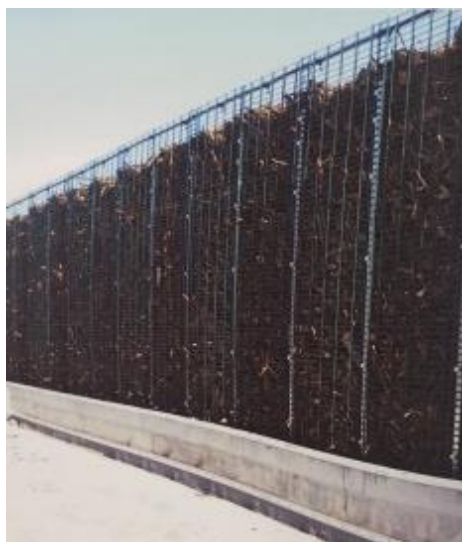
Figure 14: Photo by Author of Display at Farm Appreciation Day, Germany. Particulate filter for dust made of mesh and mulch type of material.
