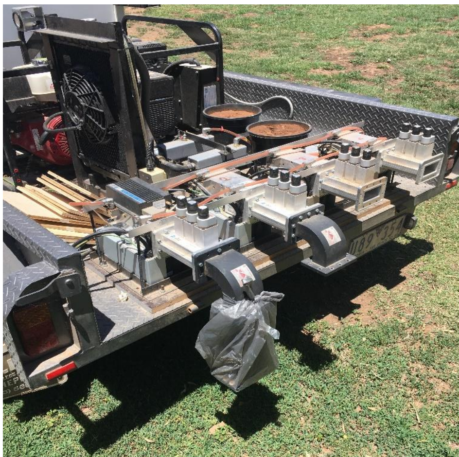
Figure 15: The back of the prototype microwave machine complete with 4 applicators.
