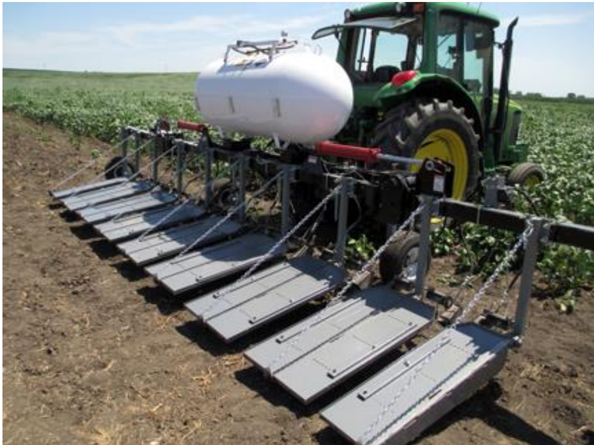
Figure 12: Showing a hooded inter row flaming machine complete with fuel supply tank
