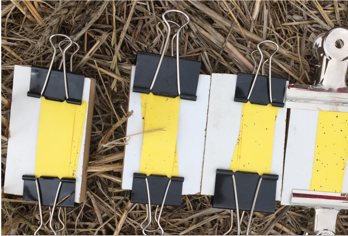
Figure 11: An image of applied rates of 0%, 25%, 50% and 100% of prescribed rate applied to water sensitive paper at random points across the boom. (Top papers only).
