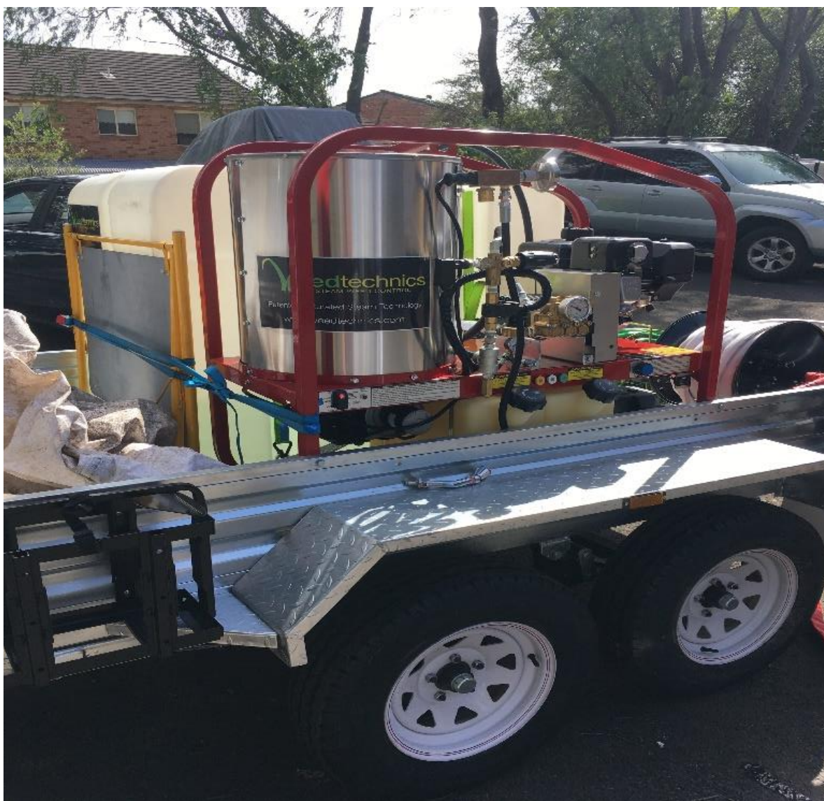
Figure 14: Weedtechnics small scale rig for handheld applications along with the applicator.
