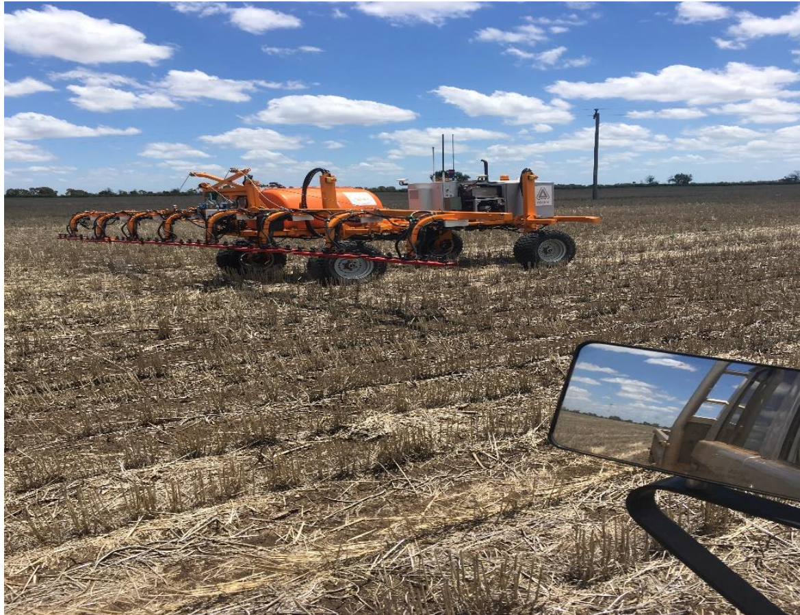
Figure 18: Swarm Farms' fully autonomous spraying platform.
