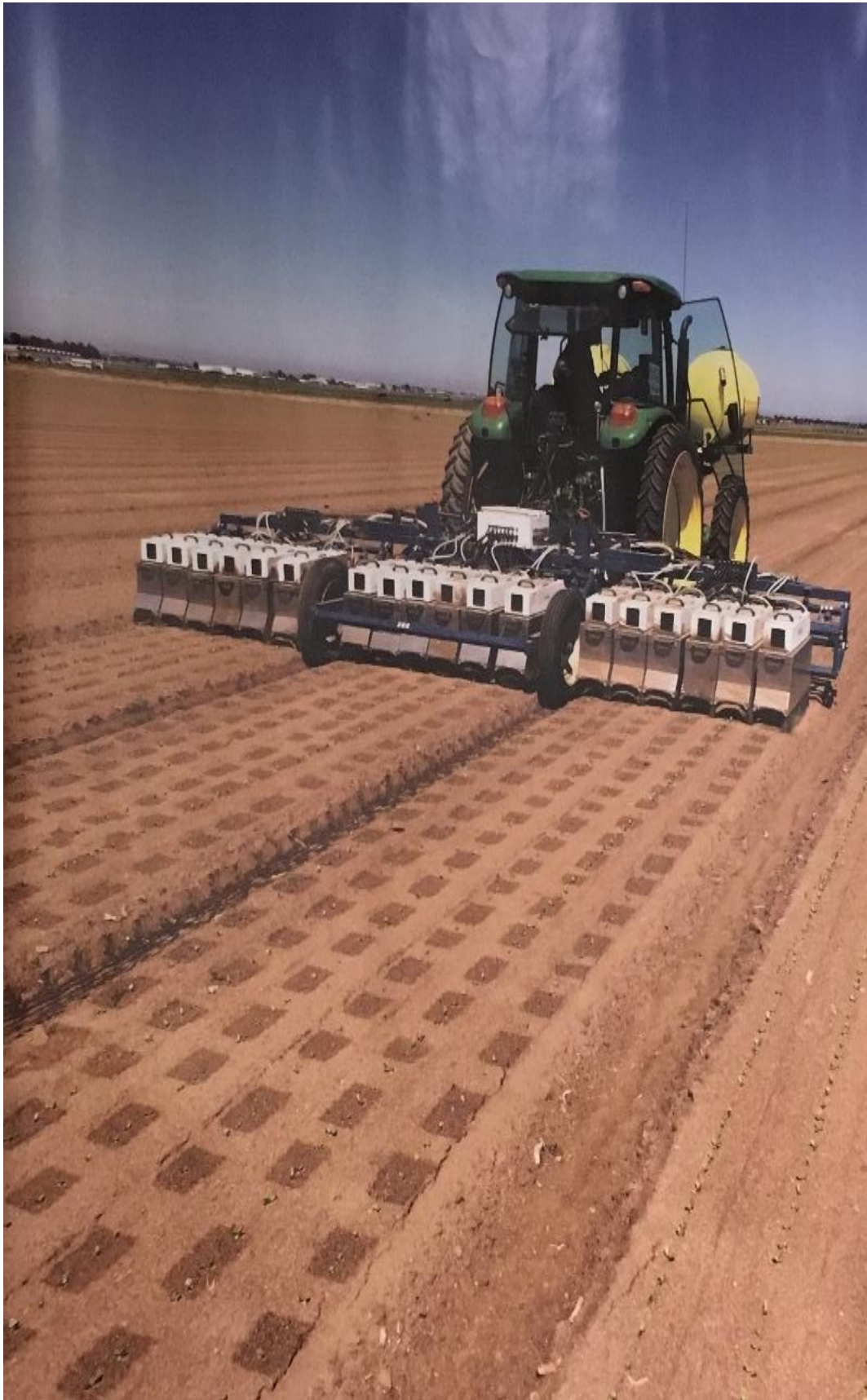
Figure 10: Blue River Technologies automated thinning machine
