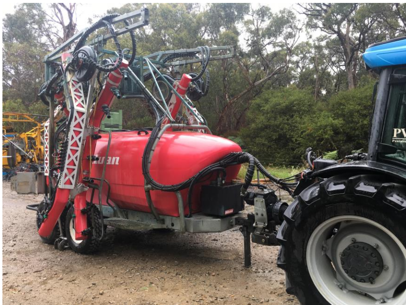
Figure 6: A 3 row, 3,000 litre vineyard sprayer on Mornington Peninsula, Australia
