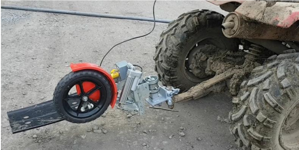
Figure 10: Viewing the Jenquip rapid plate meter on trial in Cork, Ireland (Source: Author 2017)
