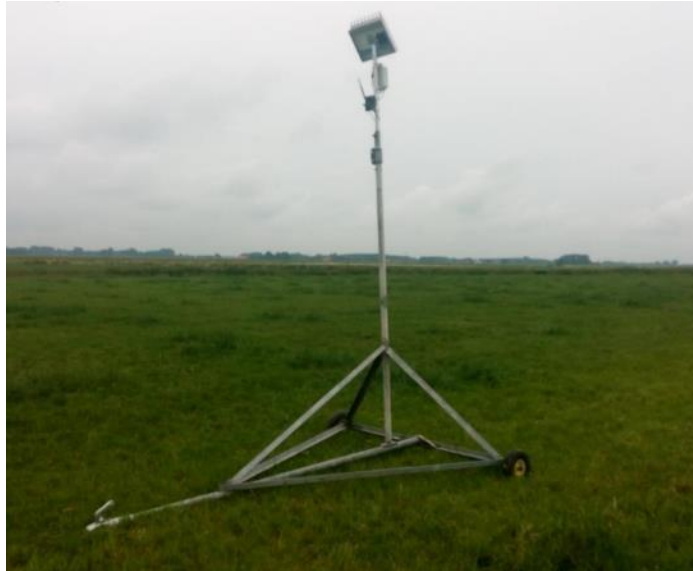
Figure 3: Mobile receiver for Cow Manager system allowing relay of cow information when cows in a grazing situation are out of range of the dairy. (Author, Netherlands, 2016).
