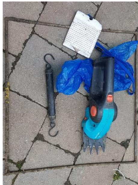
Figure 8: A pasture measurement kit including quadrat, clippers and weigh scale with conversion chart viewed on farm in Northern Ireland (Author, 2017)
