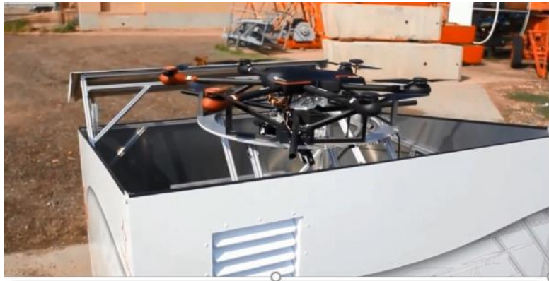
Figure 14: Autonomic drone platform by Cattlewatch (CattleWatch, 2017)
