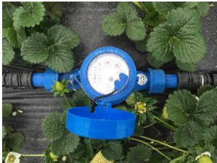
Figure 61: Simple water meters to monitor usage (Author)
