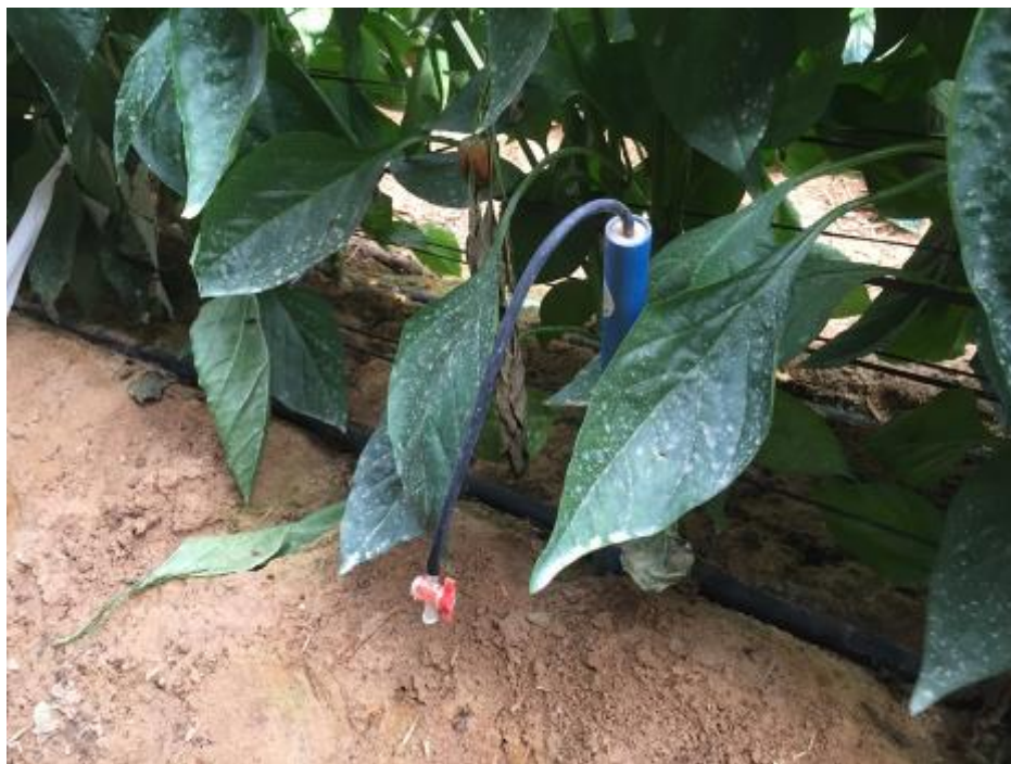
Figure 42: Lysimeter installed in a capsicum crop (Author)
