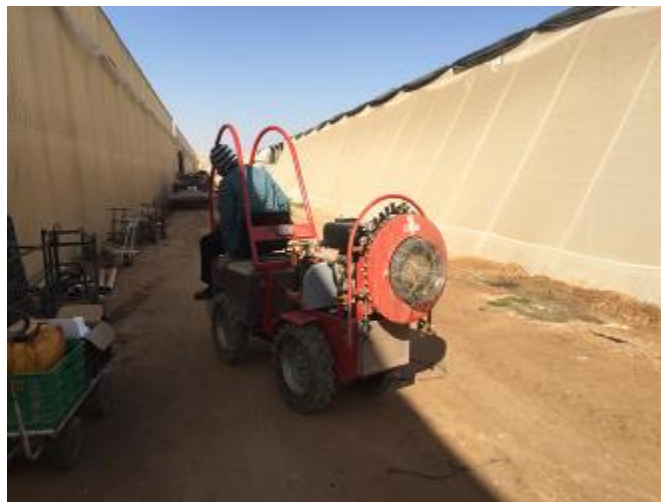
Figure 46: Diesel driven 4WD sprayer, it can drive between the rows and spray using fans
