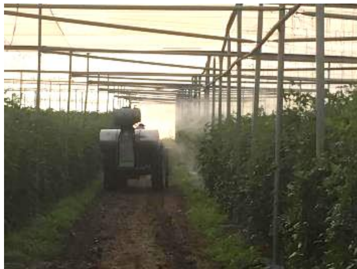
Figure 47: Canon sprayers behind tractors blow 25m down a row for preventive spraying
