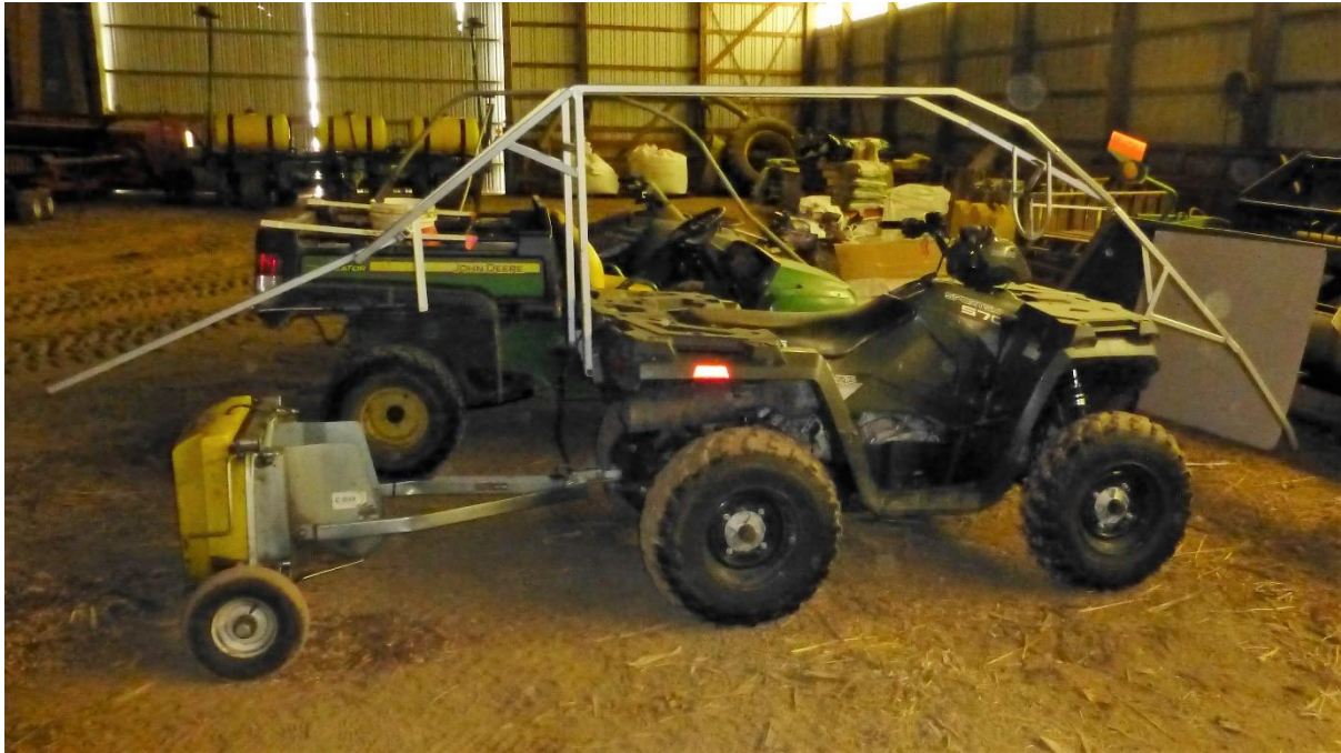
Figure 4: Modifications made to an ATV to facilitate grass observation, at the W K Kellogg Biological Station, Pasture Dairy Center
