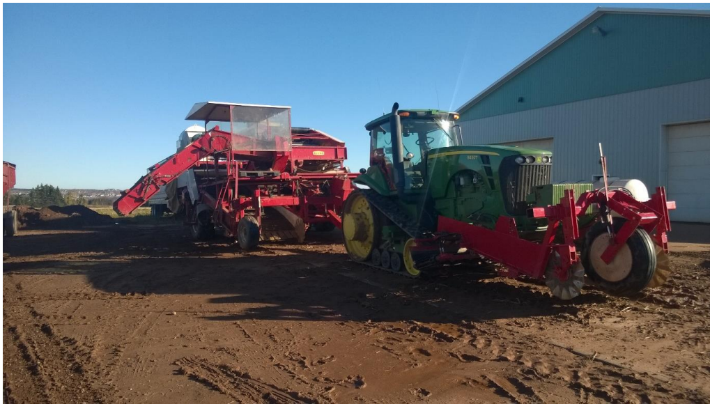
Figure 27: When combined with 6-row windrowers, harvesters like this at Rollo Bay Holdings on Prince Edward Island can harvest over 8 Acres/hour.
