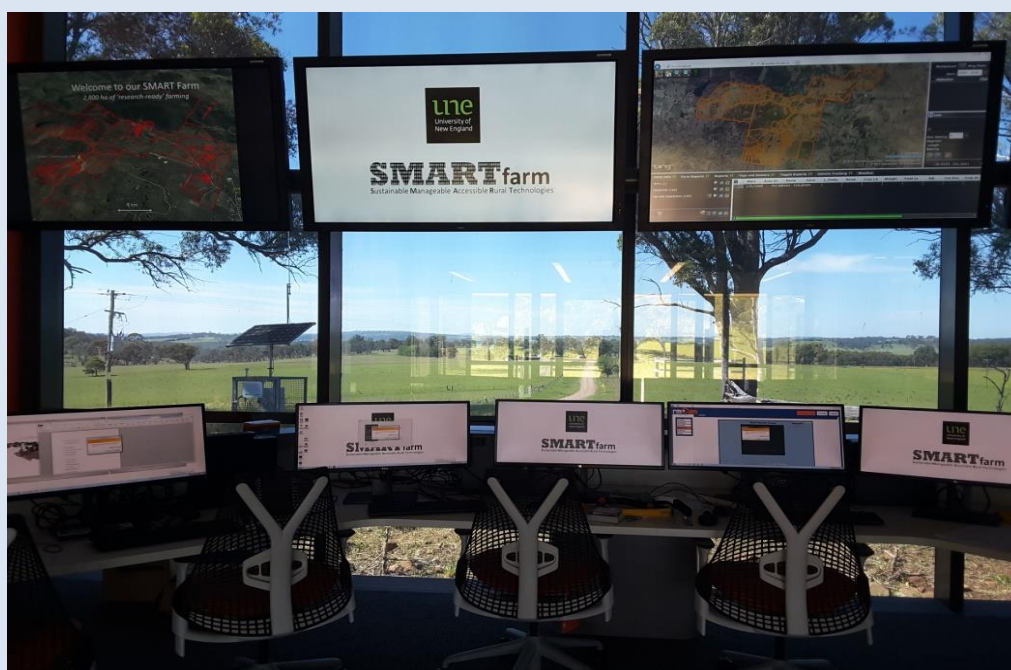
Figure 7: Data management centre at UNE's SMART farm hub. Live feeds of soil, plant and animal sensors can be viewed here and tools such as pasture growth forecasters used to help manage the grazing platform.
