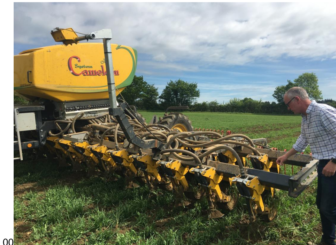
Figure 55: System Cameleon drill. Once drilling the crops is finished, the machine can soon be changed into an inter row hoe. (Shimpling Park, Suffolk, UK)
