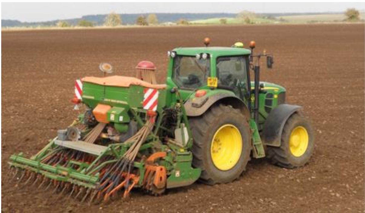
Figure 47: The power harrow combination, a farm favourite during the 1970s, 80s, 90s and well into the 2000s. Maximum soil disturbance by mechanical stirring.
