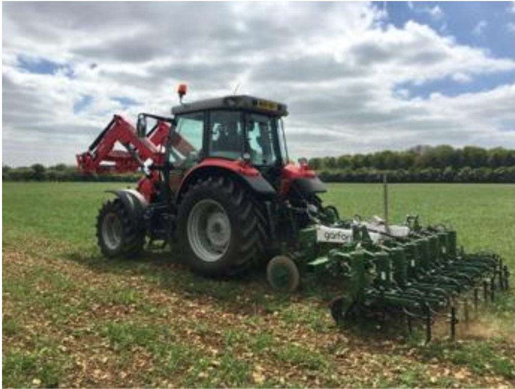
Figure 53: Robocrop guided hoe as demonstrated by George Hall, at Mechanical Weeding Live (Rural Innovations Centre, RAU Cirencester)
