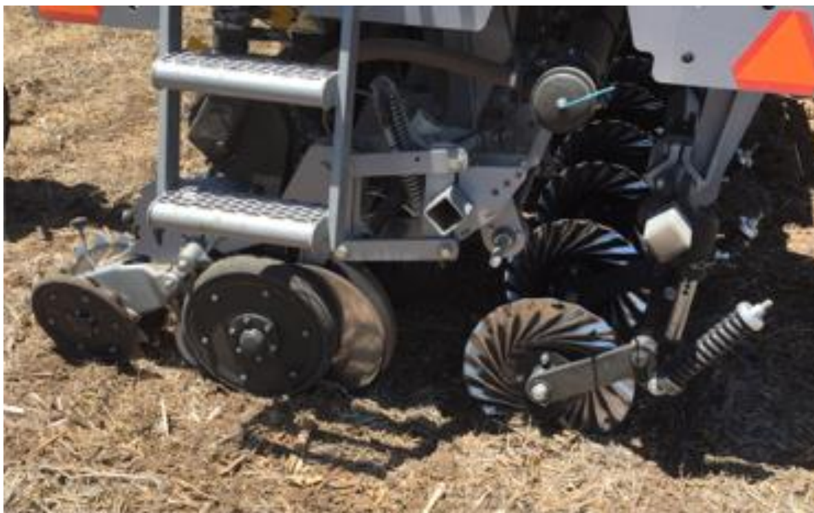
Figure 49: Minimum disturbance disc drill used in San Jose Uruguay - used the world over in no tillage agriculture and fast becoming popular in the UK.
