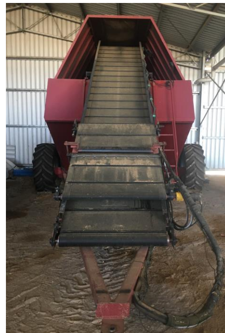
Figure 31: Chaff cart and elevator. Western Australia
