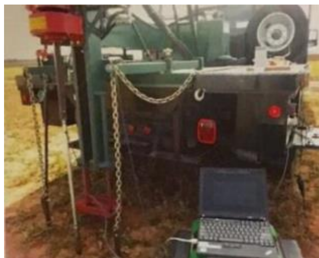
Figure 16: Penetrometer with integrated Vis-NIR Sensor (Source: Author)
