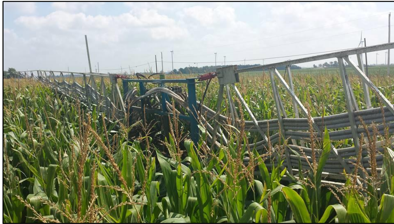
Figure 8: The Nutrient Boom traveling through standing corn while applying dairy manure. Source: Ohio State Extension Environmental and Manure Management
