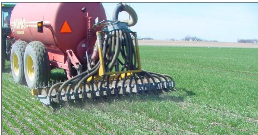
Figure 5: Manure being knifed in with a PEECON toolbar. Essentially it puts a slice in the field and the manure on top and compared it with surface applied urea as it has traditionally been done. The results were 95 bushels with the knifed in manure compared with 88 bushels for surfaced applied urea. Source:
