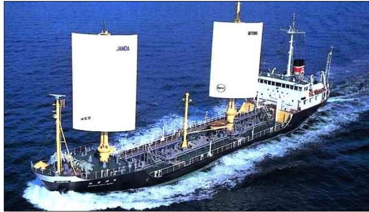
Figure 10: JAMDA - A computer controlled, sail assisted merchant ship
