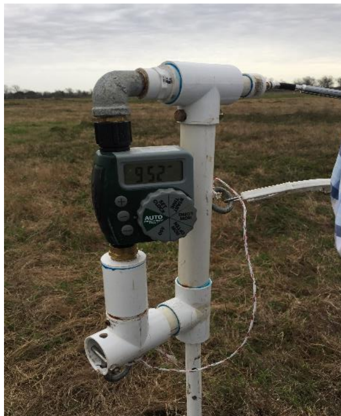
Figure 16: Pneumatic timed gate release mechanism, Hungerford TX. Source A. Coffey 2017
