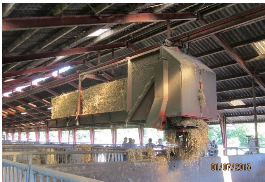
Figure 9: Automatic straw dispenser for bedding cattle, working in a 192-metre long cattle house
