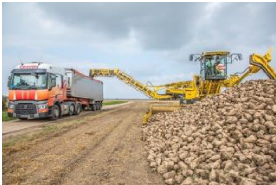
Figure 13: A self propelled cleaner loader loading a lorry
