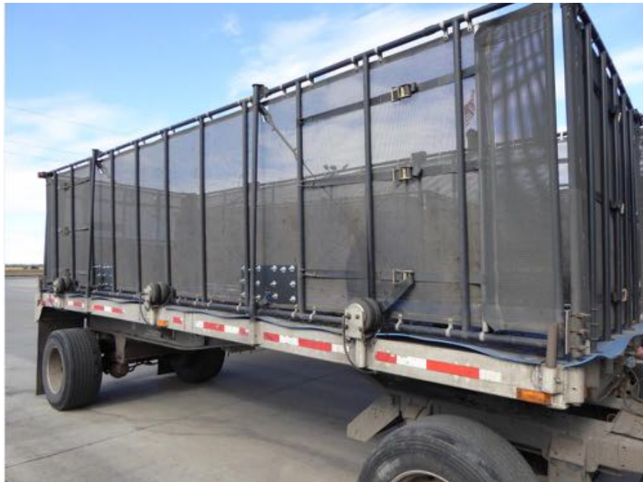
Figure 36: A mesh sided trailer used to transport sugar beet in the Red River Valley - USA
