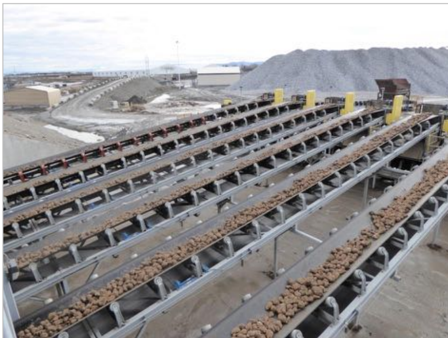
Figure 39: Showing beet handled from beet unloading to the factory via rubber conveyors in Idaho, USA
