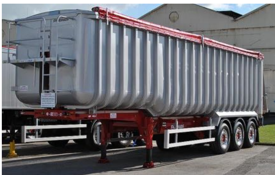
Figure 35: A typical Tri Axle bath tub Fruehauf bulk tipper
