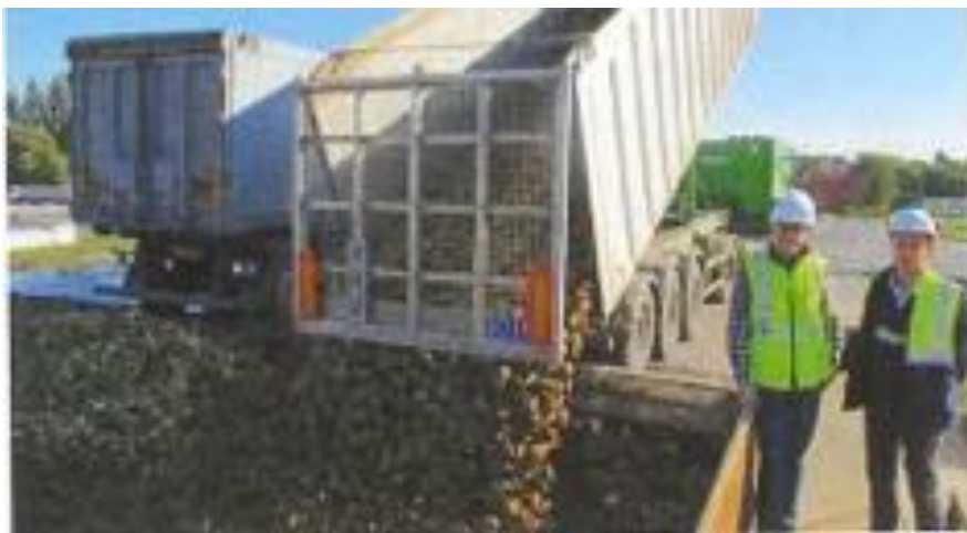
Figure 32: Figure 31 – Showing the screen gate (on the right compared to conventional on left) used by Tereros in France. ( Sugar Industry, November 2015 )
