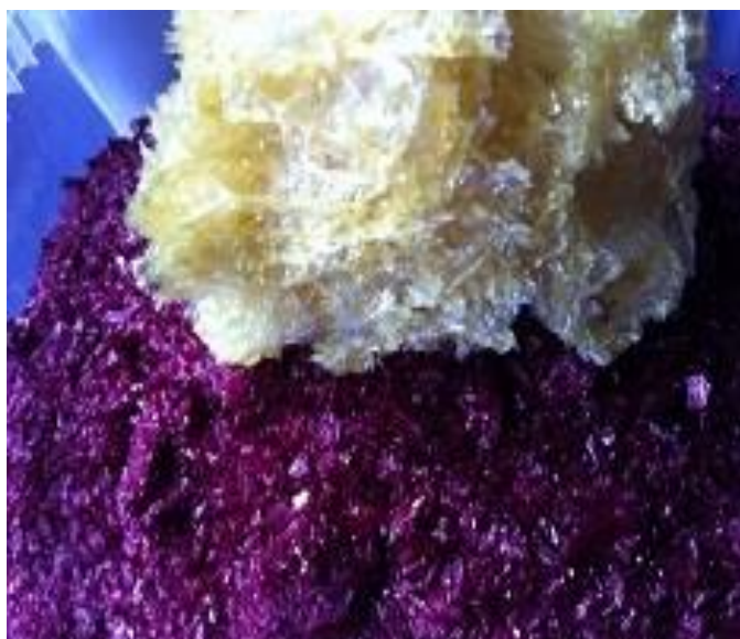
Figure 16 – Food crystals created from vacuum dried vegetable juices.
