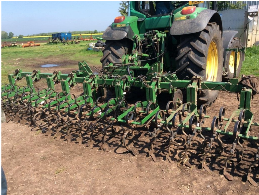
Figure 52: camera guided inter-row hoe from Garford Machinery
