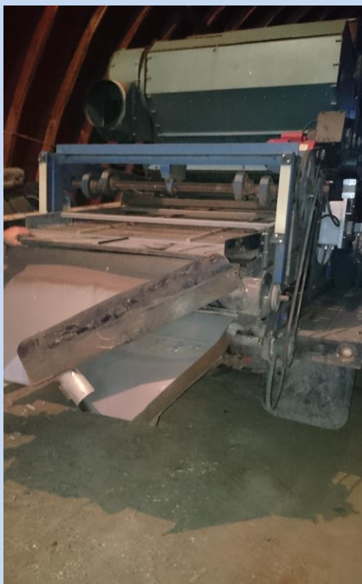
Figure 35: converted old Flaman 54" screen cleaner
