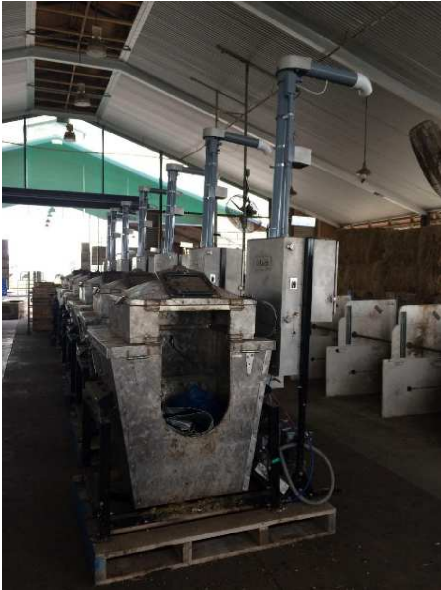
Figure 39: Apparatus to measure methane from cows
