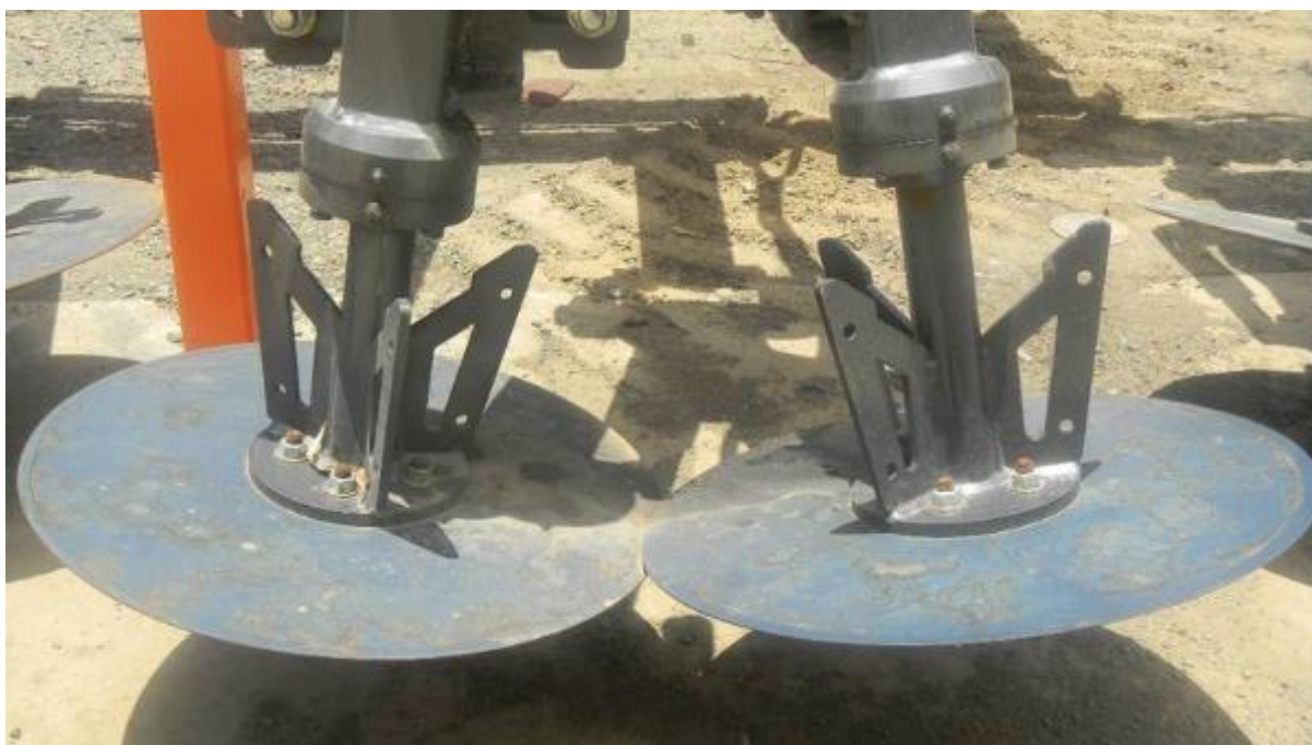
Figure 24: A Cotton Root Cutter (Source TTQ Agricultural Equipment)
