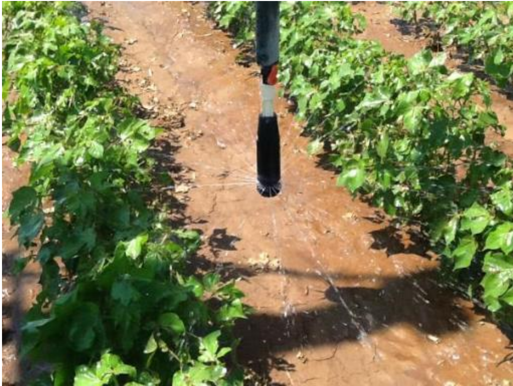
Figure 9: A Static Plate Sprinkler (Source: Author)
