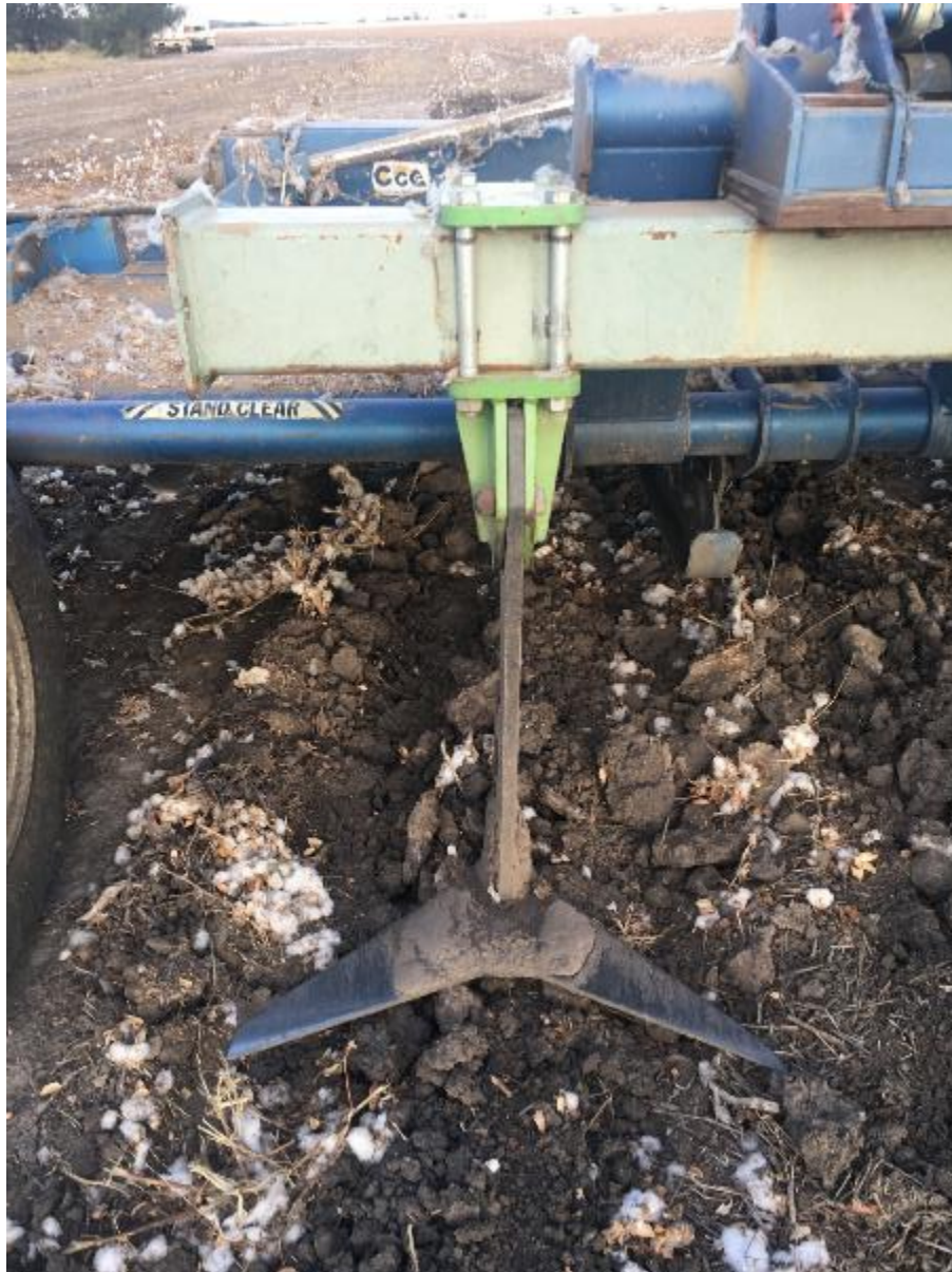
Figure 27: Rob Blatchford's slasher and shank system to dislodge cotton root systems (Source: author)
