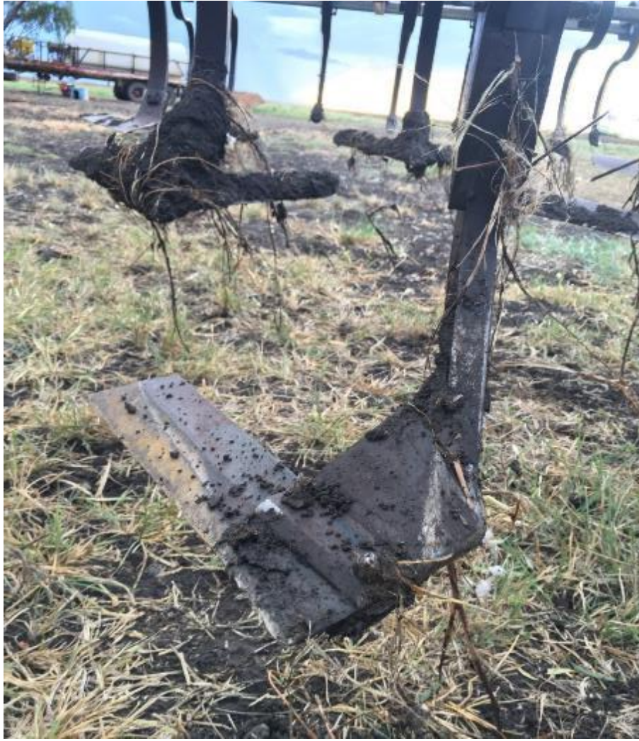
Figure 26: Jamie Grant's "knife system" to cut and dislodge cotton root systems (Source: author)
