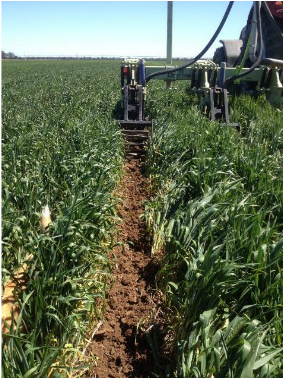
Figure 23: Preparing a fine seed bed in the plant line in a cereal cover crop using an Orthman Strip Tiller (Source: Author)
