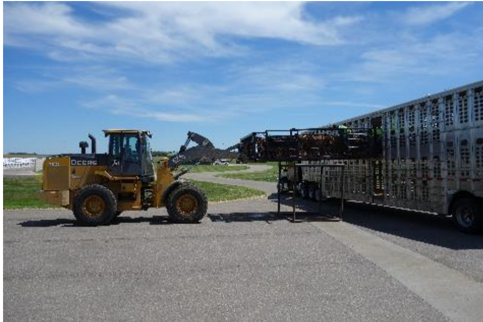
Figure 14: Loading calves onto a semi-trailer utilising a large calf pen mounted on a low-loader, Riverview, Morris, Minnesota (Source: Author)
