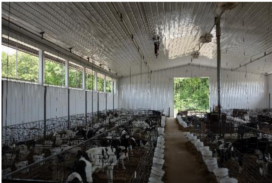
Figure 17: Barn calf rearing research facility on the Lambrights farm Shipshewana, Indiana. Calves are in individual pens which can be hoisted into the ceiling for cleaning out between batches. The barn is heated by a wood heater during winter. Calves are bedded on sawdust (Source: Author)
