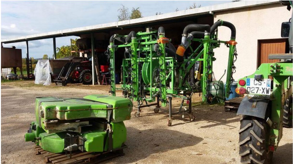
Figure 14: Specialised over-the-vine tractors and multiple row sprayers are vital in close-planted vineyards in Burgundy, France (Source: Author)
