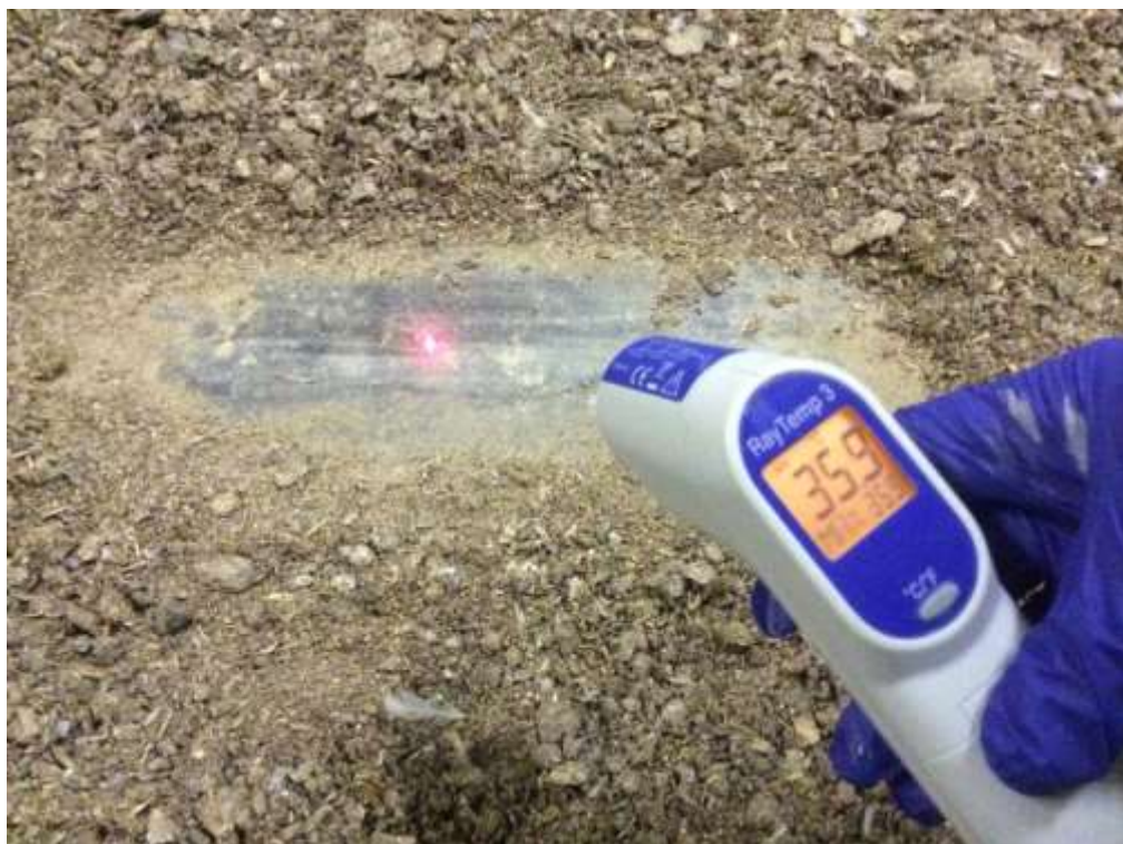
Figure 9: Underfloor heating allows shed floors to be kept very warm
