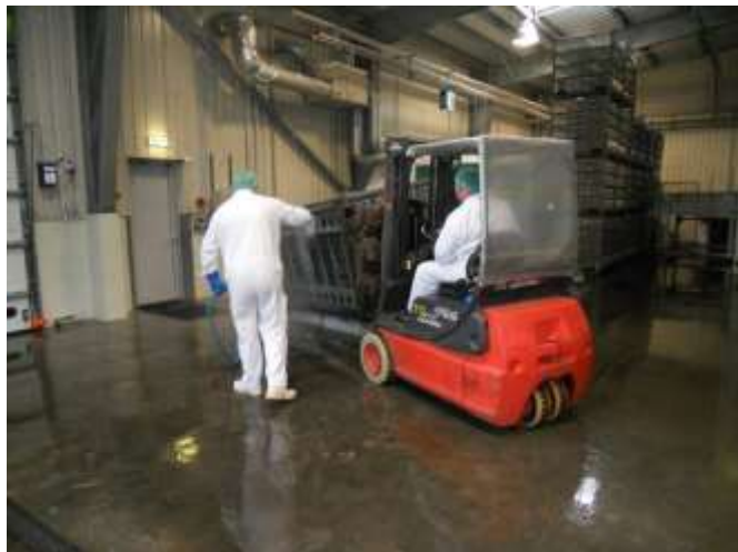
Figure 14: Crates are turned upside down to ensure that all areas are thoroughly cleaned
