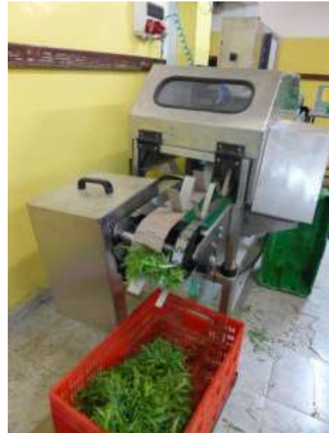
Figure 19: Herb trimming and bunching machine, for high end precision cut herbs - Jordan Valley Herbs (Israel, Nov. 2014)
