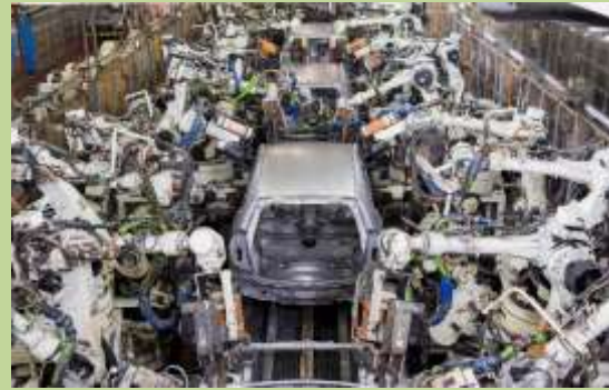
Figure 24: Spot welding robots, Toyota (Japan, Sept. 2014)
