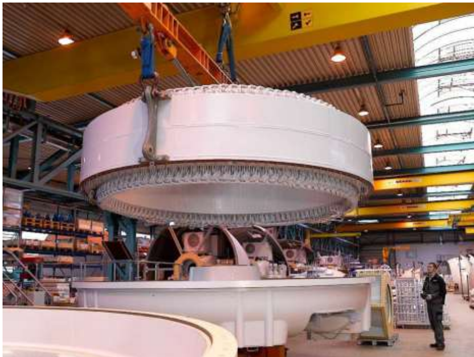
Figure 9: Enercon Factory generator assembly
