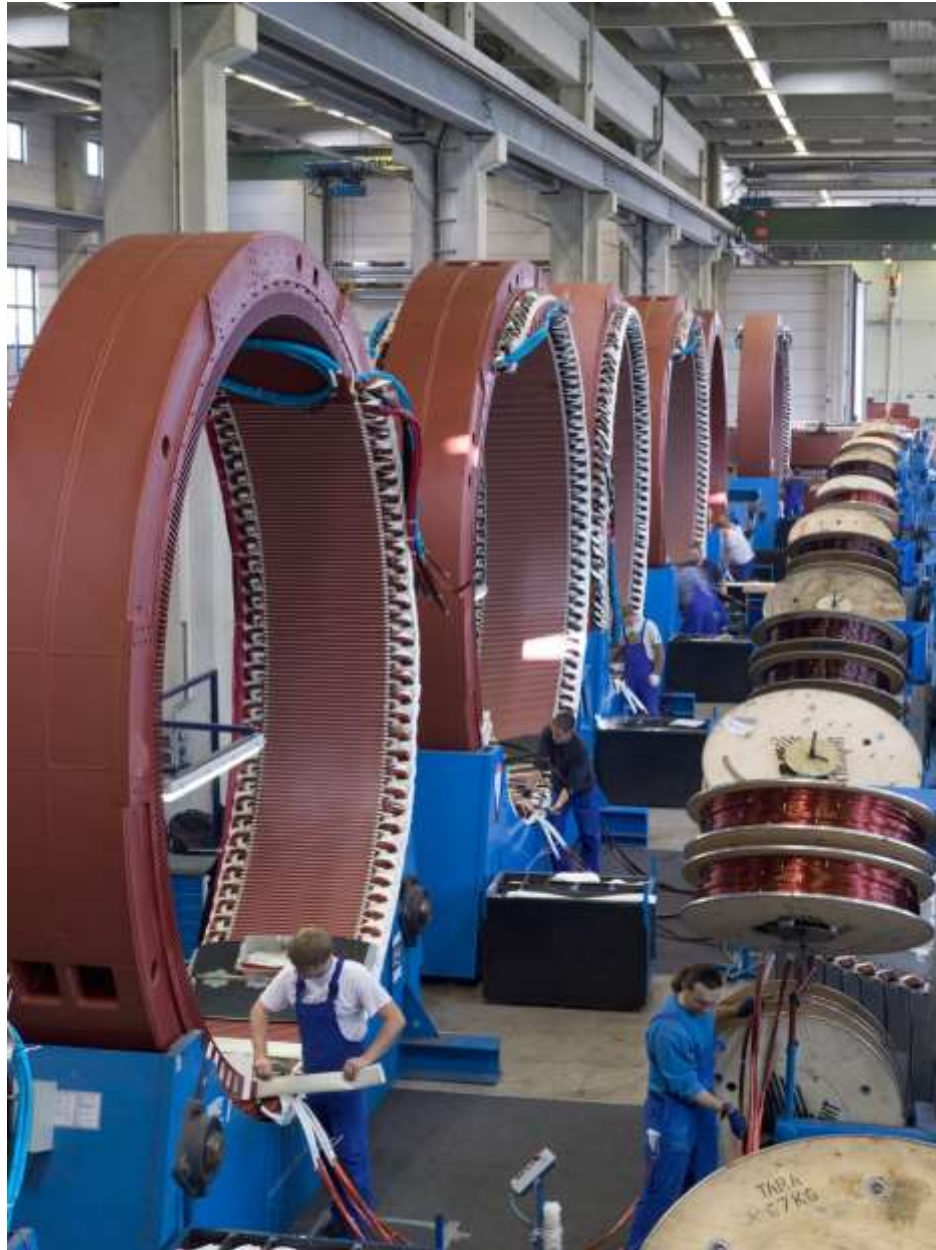
Figure 7: Enercon factory generator production line
