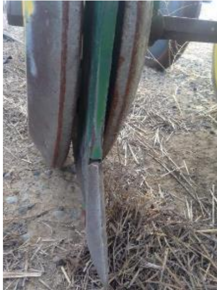
Figure 17: Deep-furrow split-packer John Deere HZ drill, Ritzville, WA, USA. Source: Gillett, N. (September 2014)
