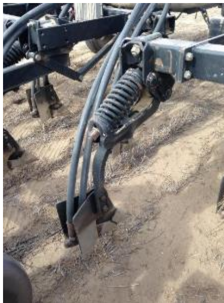
Figure 18: Fexicoil PTX drill with moisture seeking attachments. Source: Gillett, N. (September 2014)
