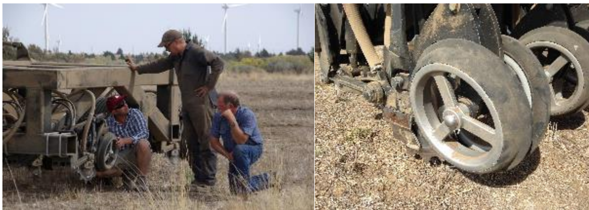
Figure 16: The author in PNW with a hybrid seed drill and a New Zealand made Cross-Slot assembly on a locally produced Ag Pro frame. Source: Gillett, N. (September 2014)
