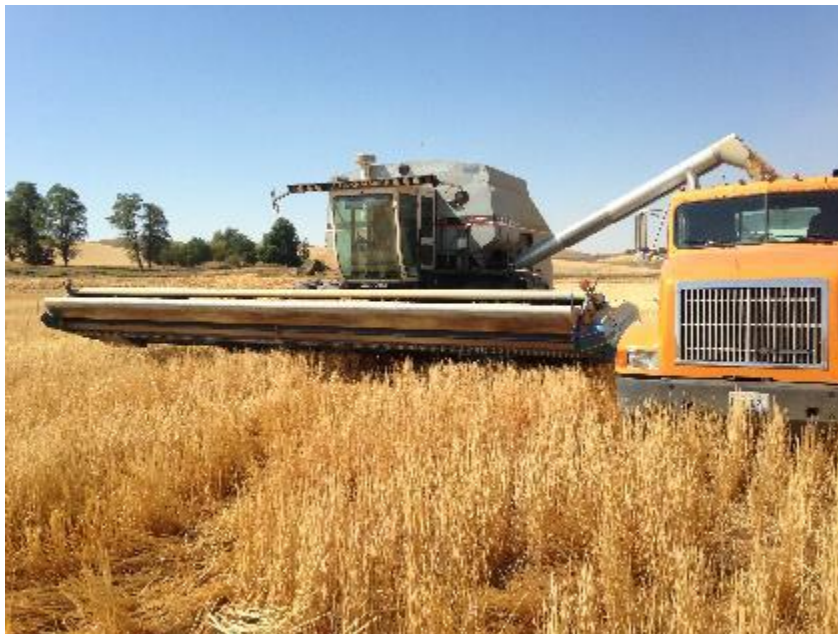
Figure 15: Harvesting with a stripper front in the Palouse, Washington State, USA. Source: Gillett, N. (September 2014)
