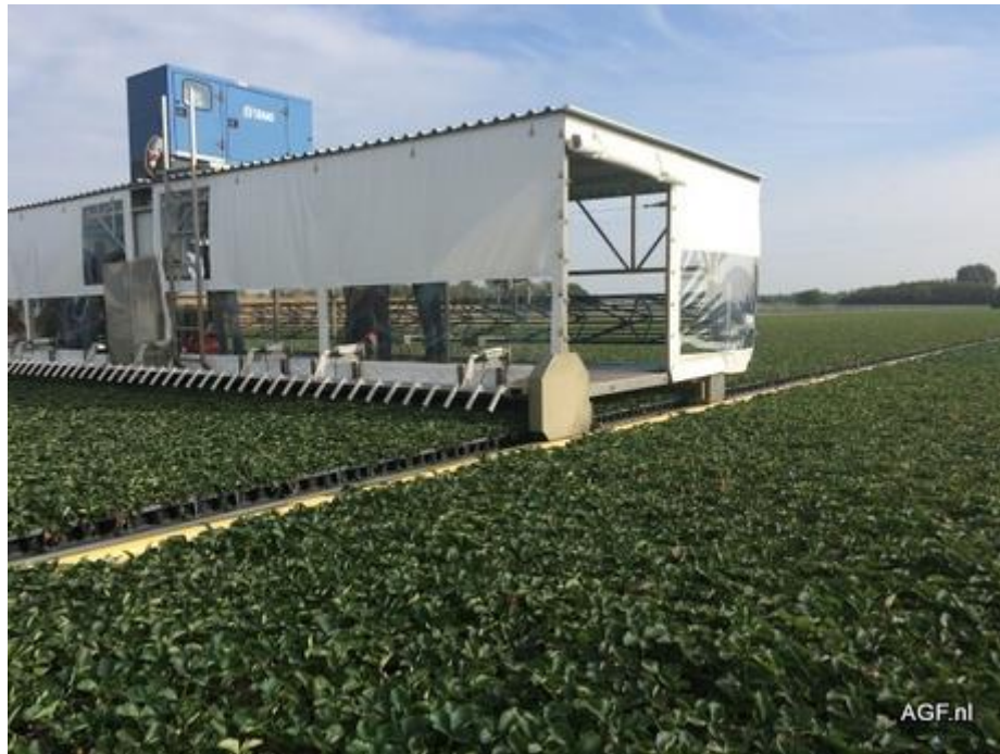
Figure 9: A platform that ‘floats’ above the strawberries allows growers to perform several operations in a protected environment (Source: Photograph courtesy of Hortdaily)
