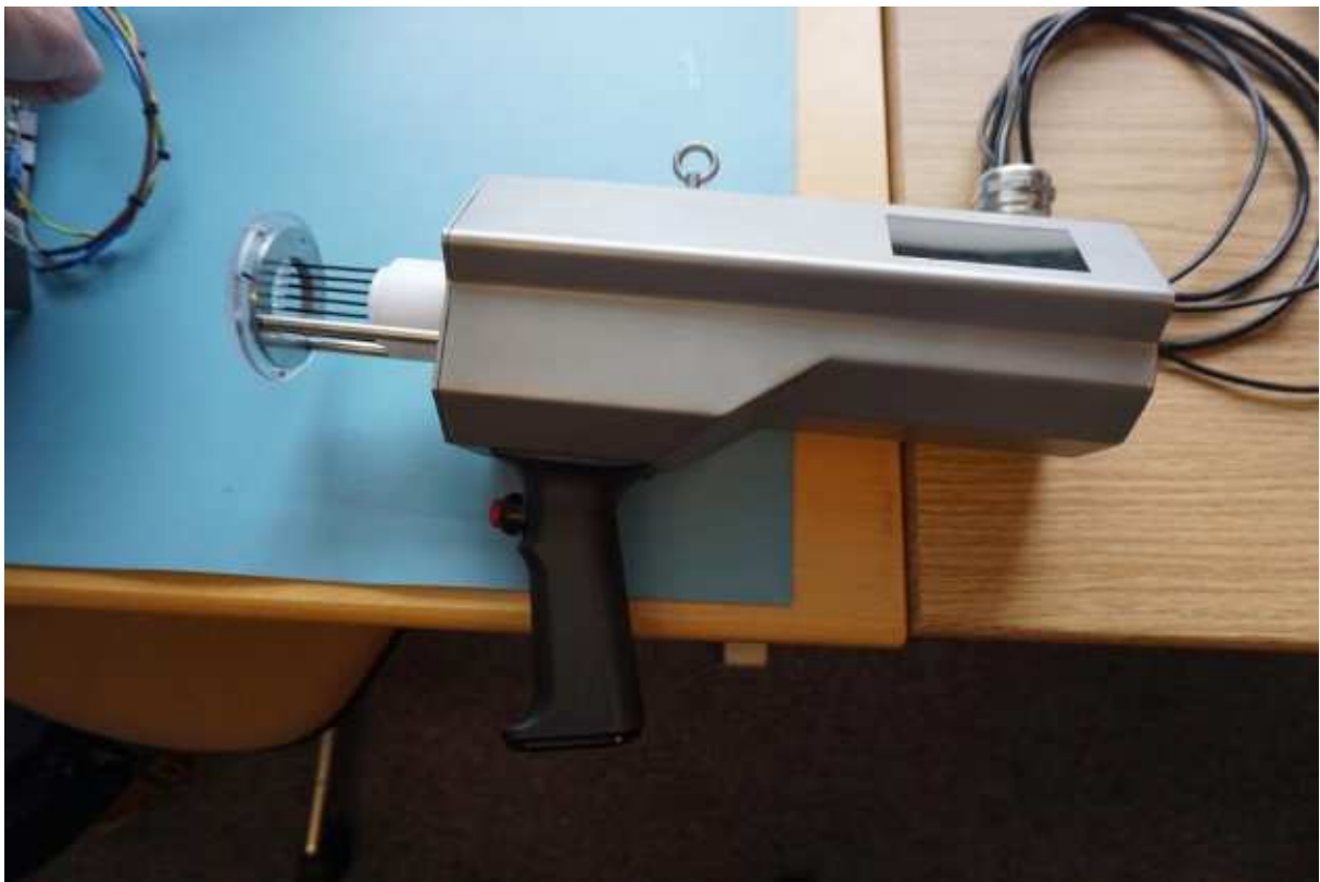
Figure 15: Fatometer under development at Carometec, Denmark. This will measure IMF through electrical conductivity and is being designed to be used in line during processing (Source: Carometec, October 2014).
