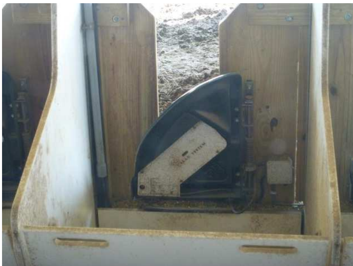
Figure 3: EID reader on feed bunks to measure daily intake is linked to weight gain to achieve a feed efficiency value (Source: Nebraska State University, April, 2014).
