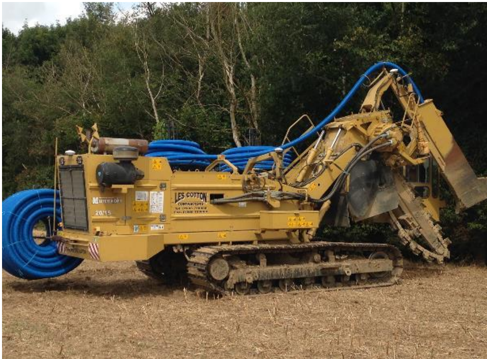
Figure 10: Mastenbroek chain trencher.
