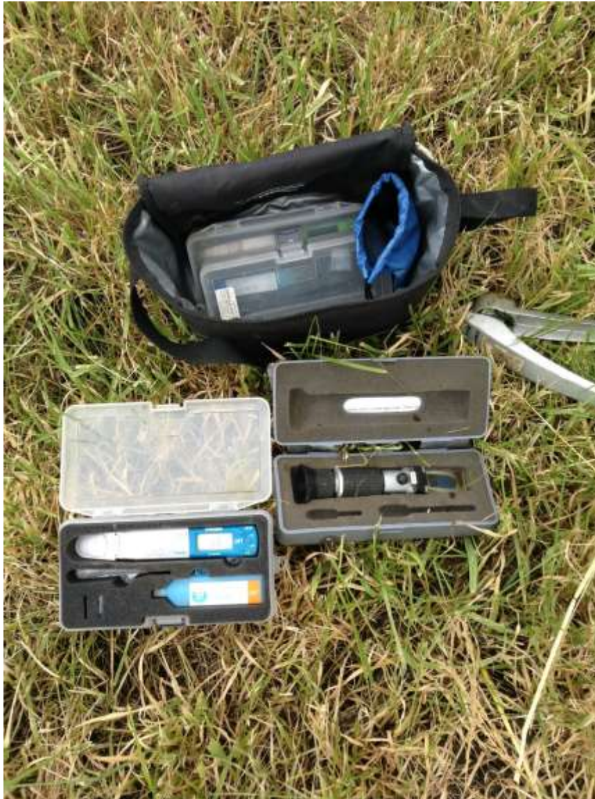
Matt Mahoney's refractometer to measure the Brix in his sward
