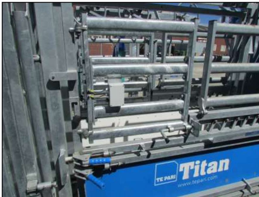
Figure 22: Antenna to read RFID tags incorporated during the manufacture of the cattle crush
