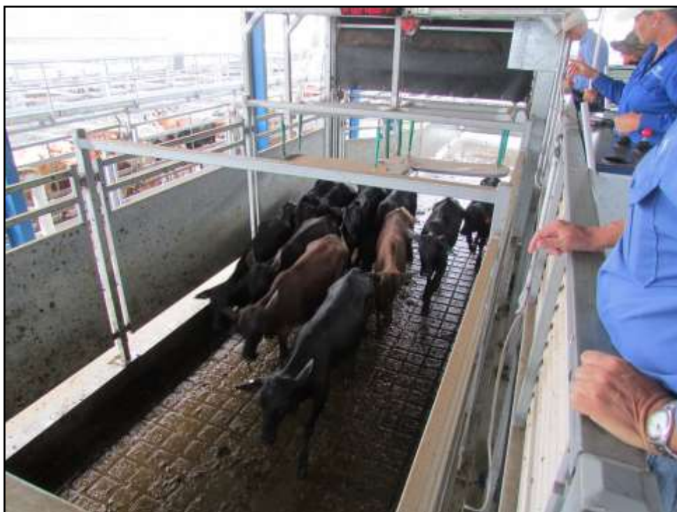
Figure 17: Weigh-bridge with RFID reader panels above the animals
