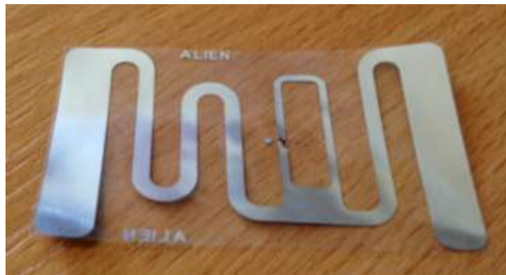
Figure 4: Ultra High Frequency chip used in cattle ear tags
