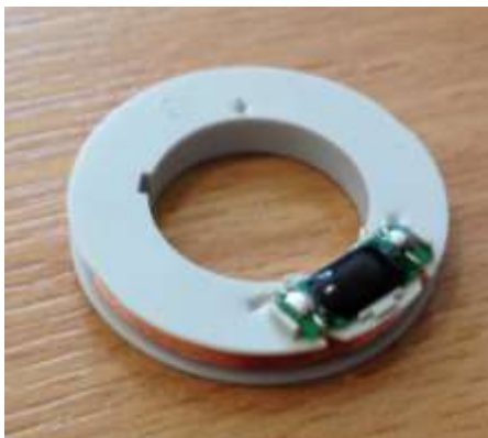
Figure 3: Low frequency Half Duplex chip used in cattle ear tags
