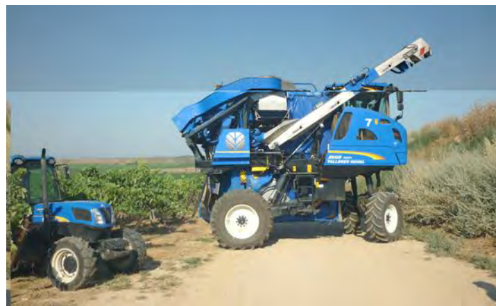
New Holland harvester capable of selective harvesting
