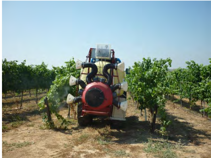
Variable rate pesticide application carried out using processed LIDAR data
