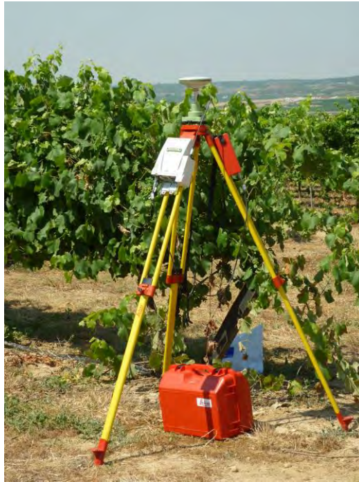
A stand-alone base station
