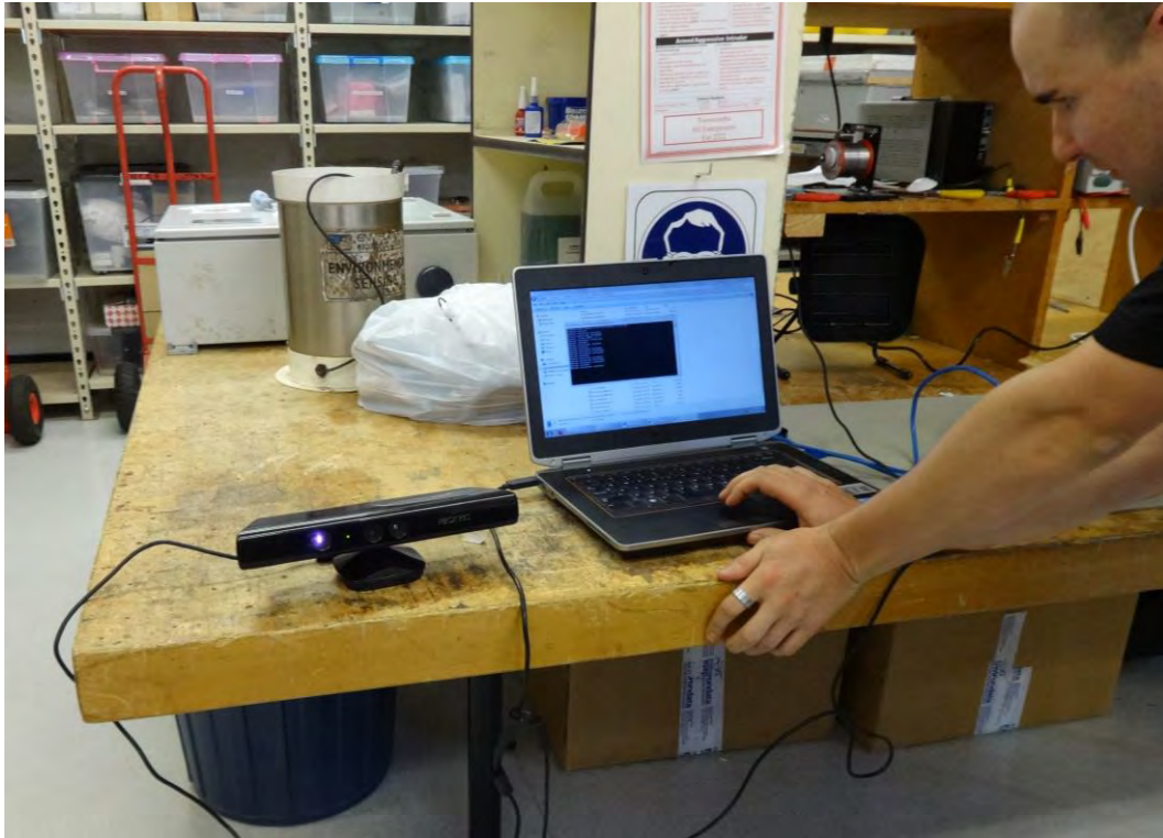
Kinect X box games console sensor used for 3D imagery and weight assessment of livestock
