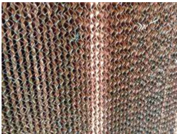
Close up of the cooling pad material and Wayne showing the constant flow of water – dripping from his elbow
