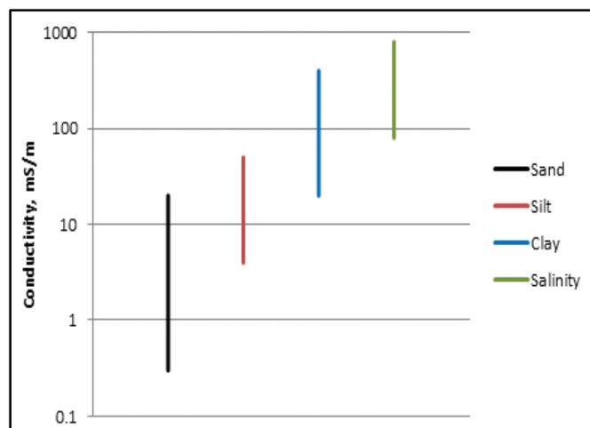
Electrical conductivity of different soil materials
