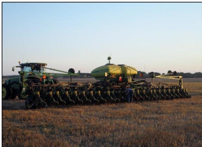
Passive implement steering system with a GPS receiver on the planter
