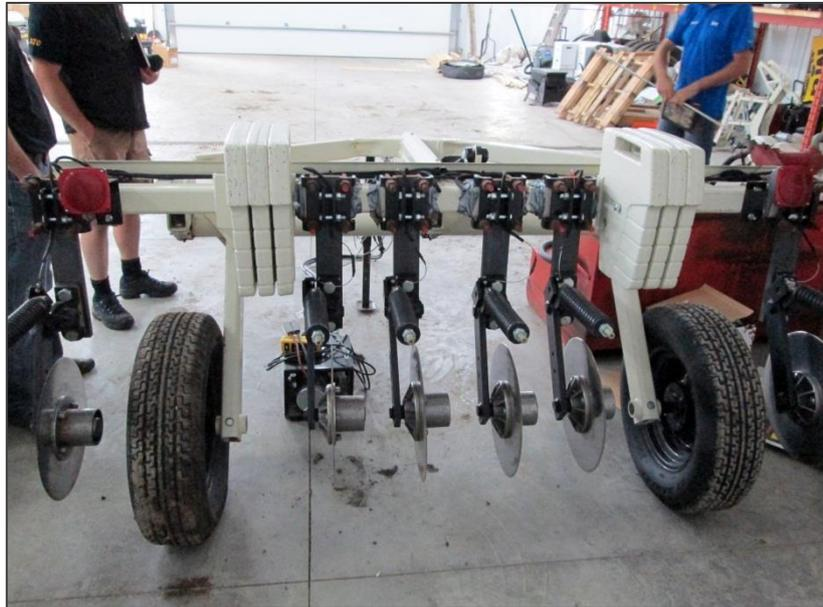
Veris Machine for measuring EC
