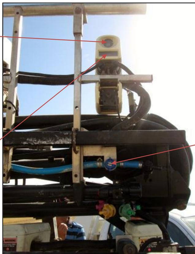
The reflected light detected is analysed and if it matches the light reflected from a green plant the fast fire solenoid is activated to only spray the plant. The sensor has the capability to detect plants from approximately 7cm upwards in diameter
