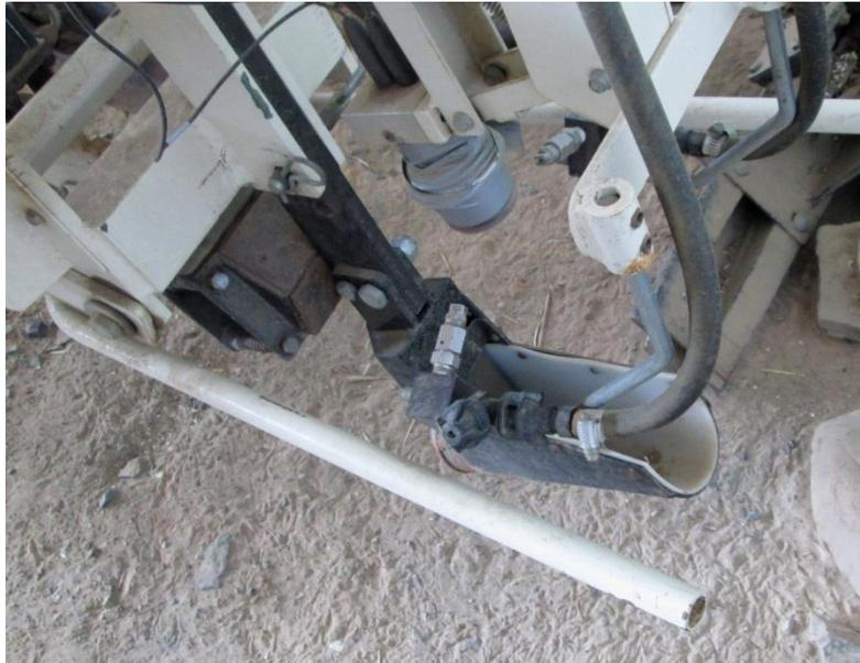
Soil sampling shoe with pH electrodes above
