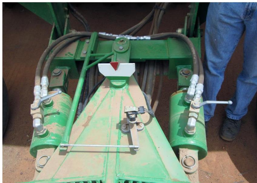
Hydraulic rams fitted to a drill drawbar
