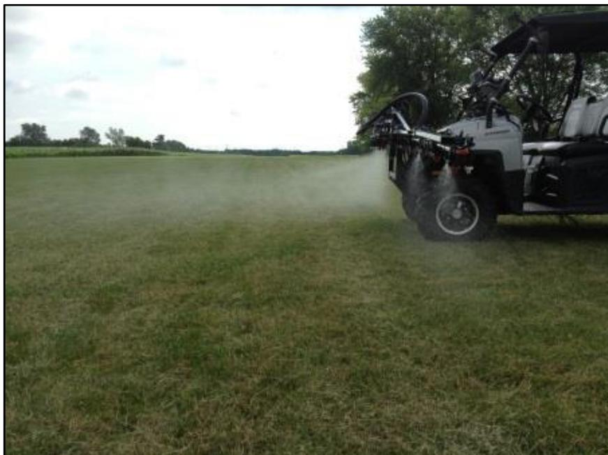
Reduced drift of PWM (near side of boom) compared to a traditional flat fan nozzle (far side of boom) at the same rate and pressure.
