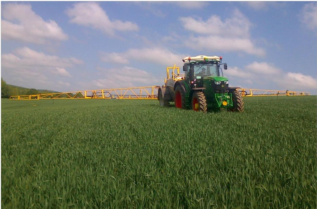
Our own tractor and sprayer working in a field of wheat, using auto steer, sectional control, auto boom height control and recording a biomass scan using a Yara N sensor for future reference
