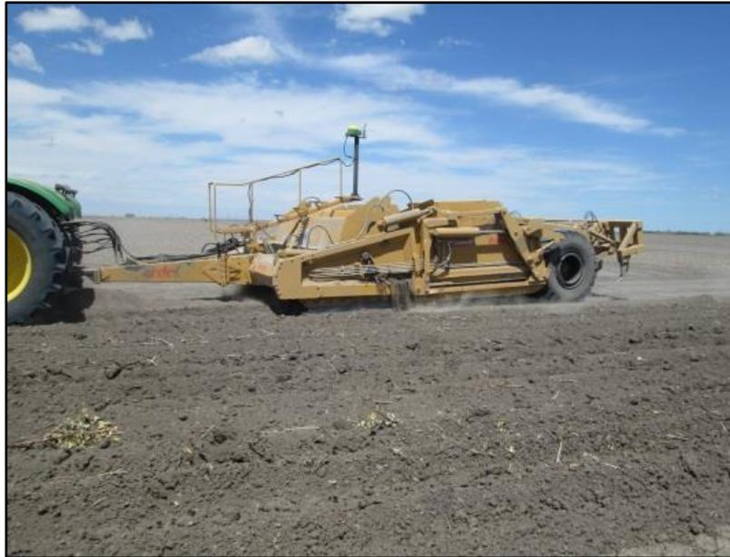
Land forming bucket using GPS levelling
