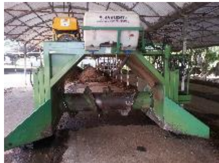
Figure 18: Compost turner, Bertrand Aubery, Martinique. Source – Inderbitzin 2013
