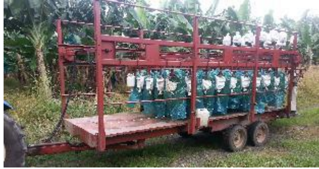
Figure 12: In field harvest trailer almost fully loaded. Source, Inderbitzin, 2013
