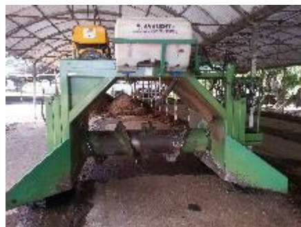
Figure 18: Compost turner, Bertrand Aubery, Martinique. Source – Inderbitzin 2013
