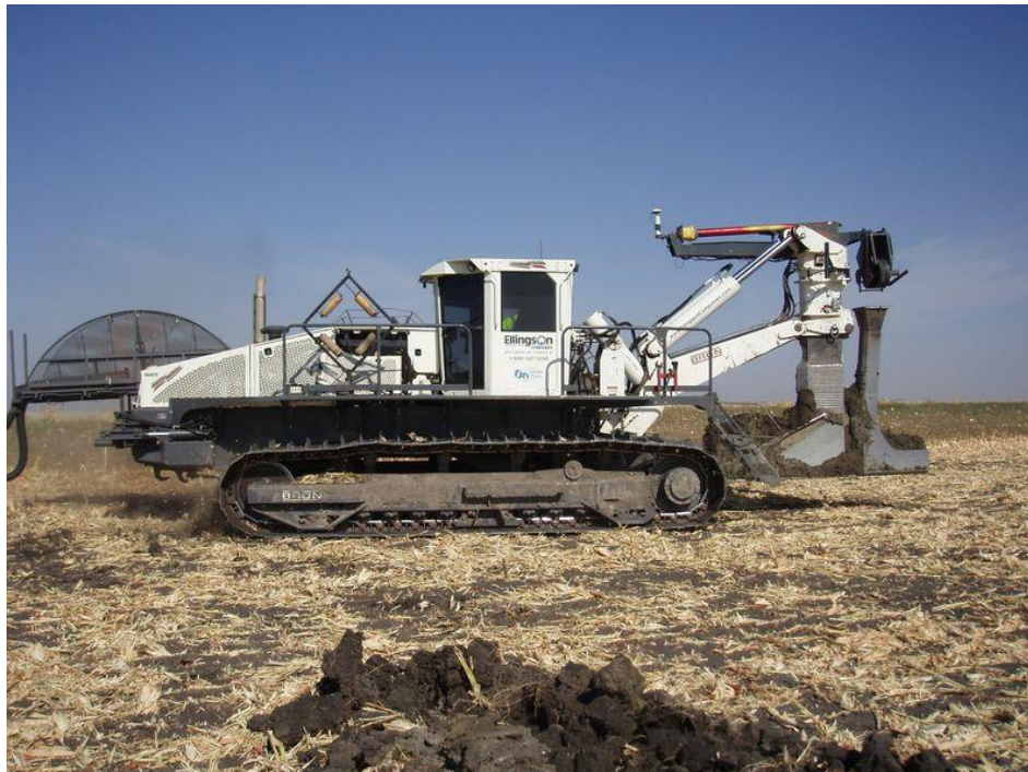
8. RWF Bron 450 trenchless drainage plough owned and operated by Ellingson Companies, USA
