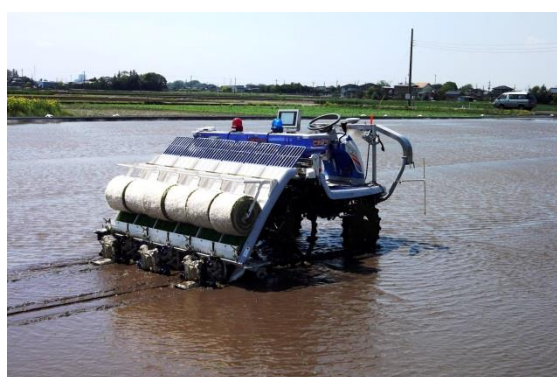
Figure 8 : Robotic Rice Planter ( NARC, Japan 2013)
