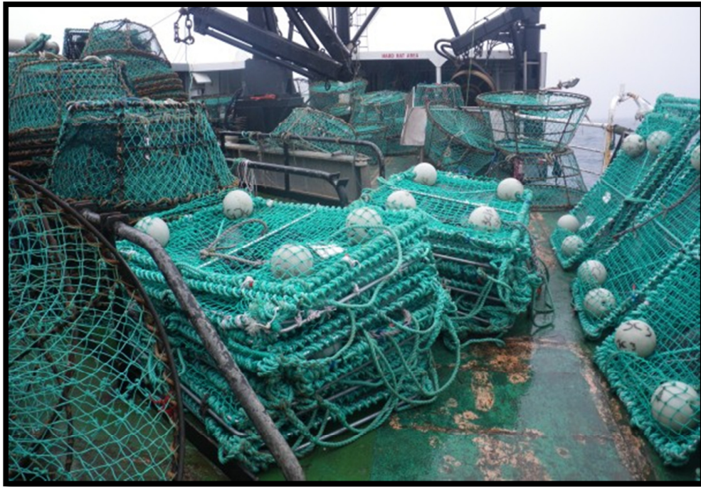
Figure 2: In the foreground, collapsible French traps. In the background, Canadian sablefish traps.
