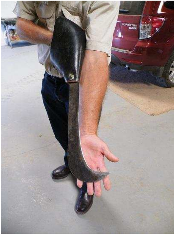
Figure 9: De-thorning knife with leather hand guard, USA 2012
