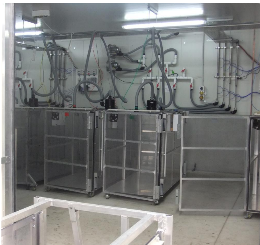
Methane measurement chambers at AgResearch Grasslands, Palmerston North, New Zealand
