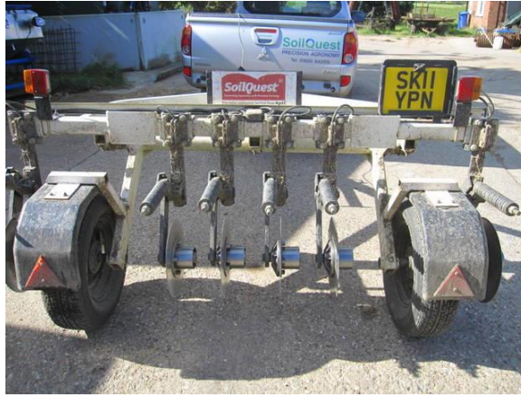
Figure 16: An example of an EC scanner (Samwell, 2012)
