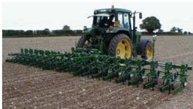
Figure 12: Garford Robocrop Precision Guided hoe, Tillett and Hague Technology Ltd
