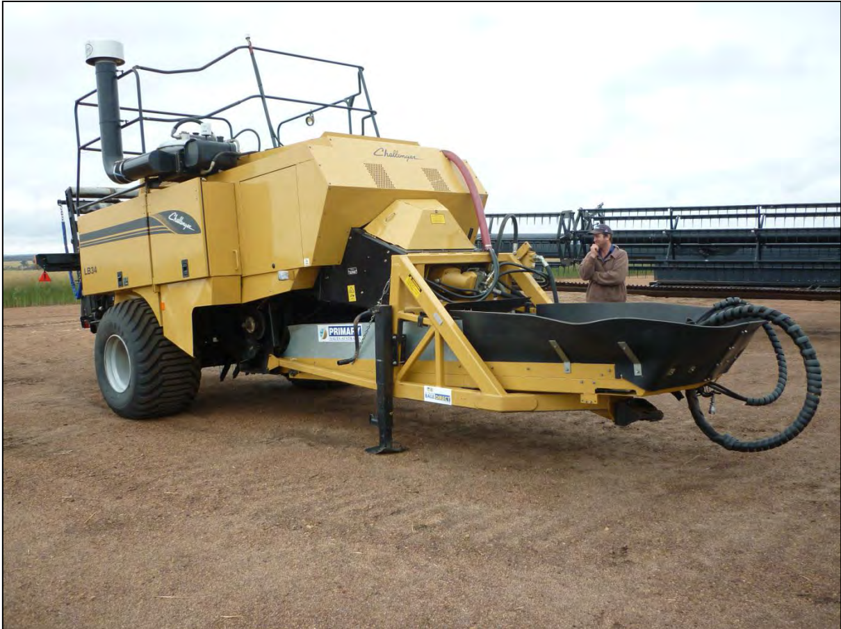
Baler fitted to the back of the combine in Western Australia
