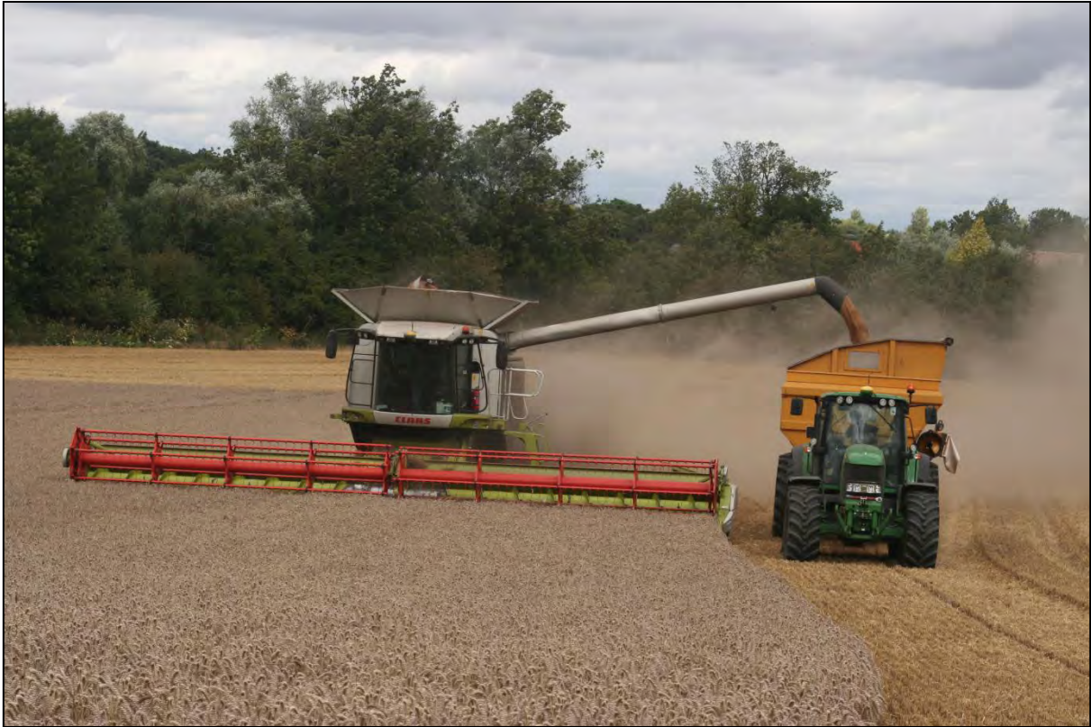
The chaser bin is compacting fresh ground due to auger not being long enough. Past combine wheeling can be seen to the right of the John Deere.
