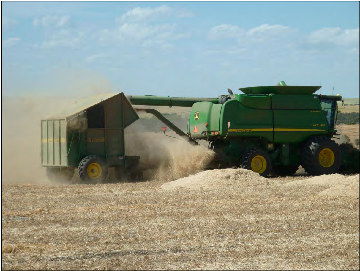
Chaff cart in operation also showing piles left on previous runs to the right of the machine
