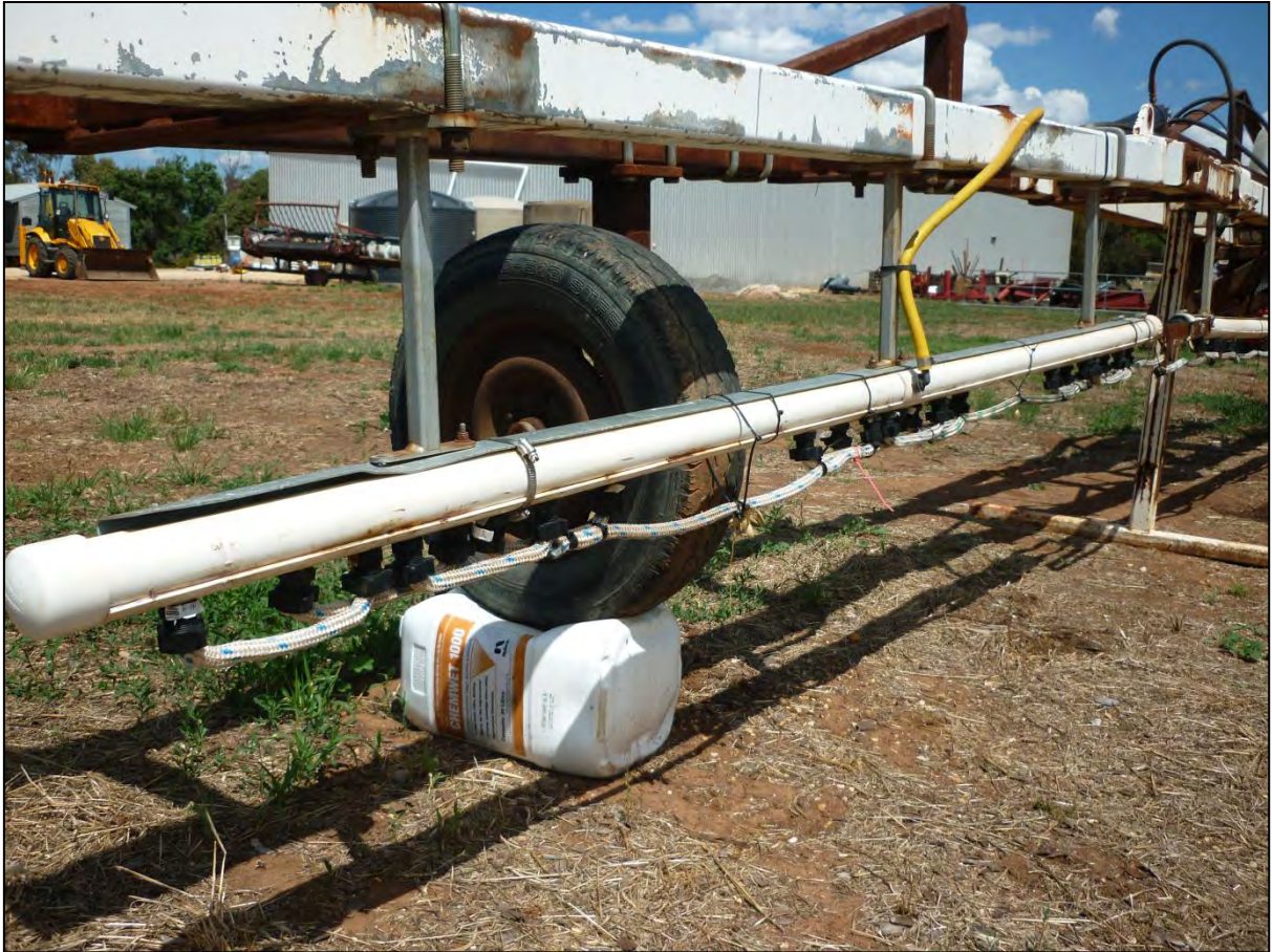
Rope charged with Roundup and used as a weed wiper
