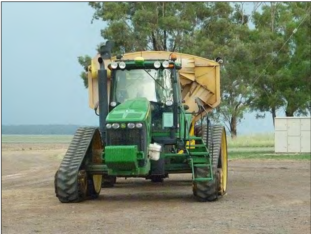
3 metre centre to centre track width
