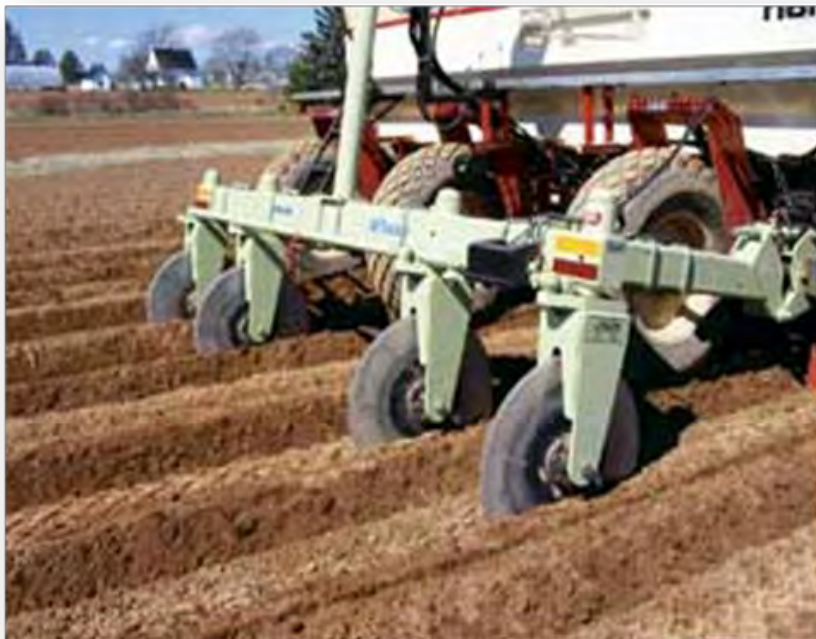
Implement being independently steered by GPS
