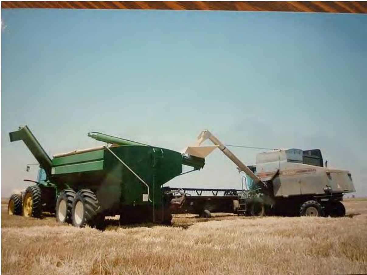
Auger extension fitted to a chaser bin.
