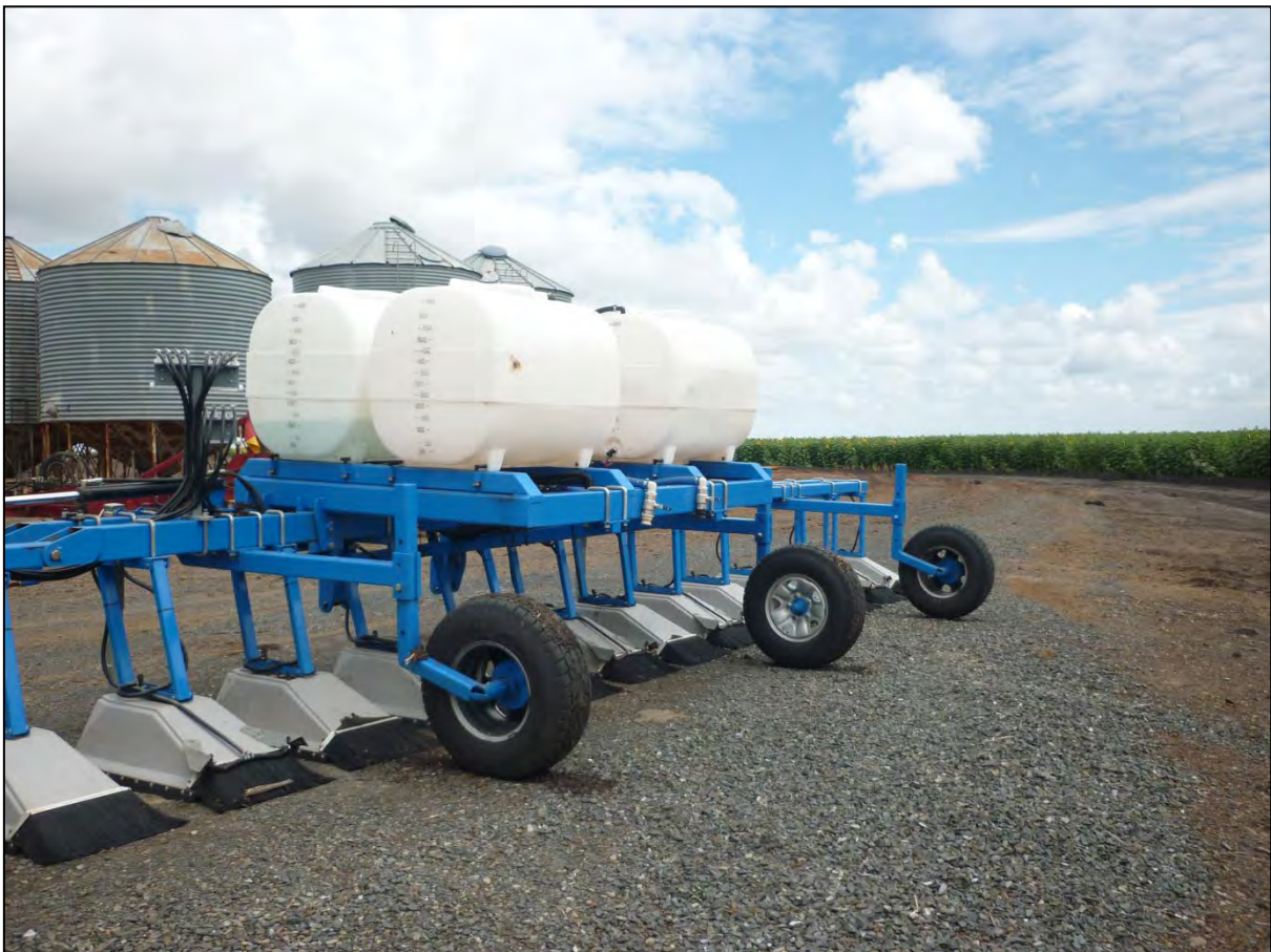
A cover sprayer able to operate between rows of combinable crops
