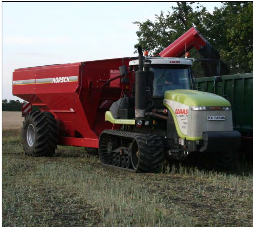
Chaser bin with hydraulic rear axle so that it can be re-aligned
