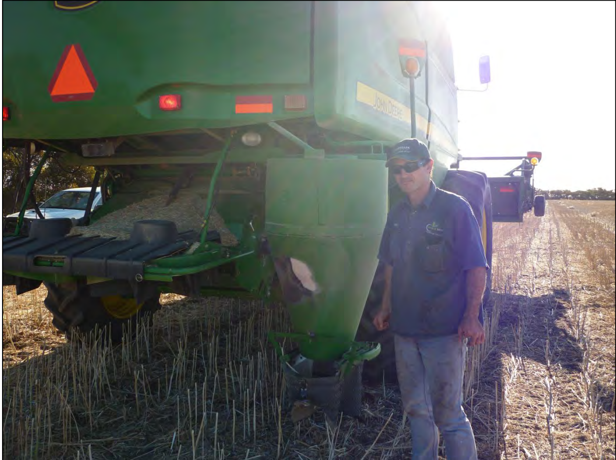
Chaff cyclone to spread weed seeds in a concentrated area directly onto the good tilth
