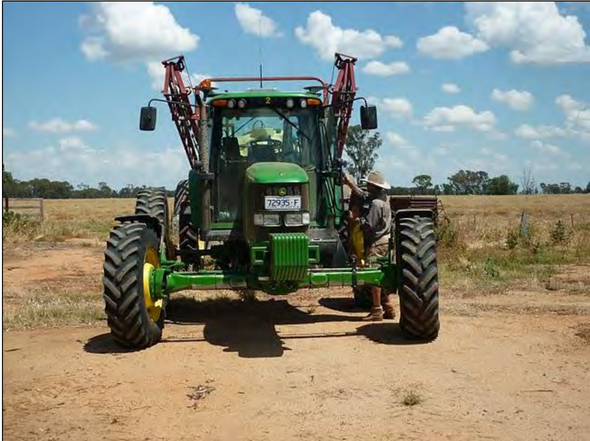
Wheeled tractor adaptation. Front axle 3 metre centre
