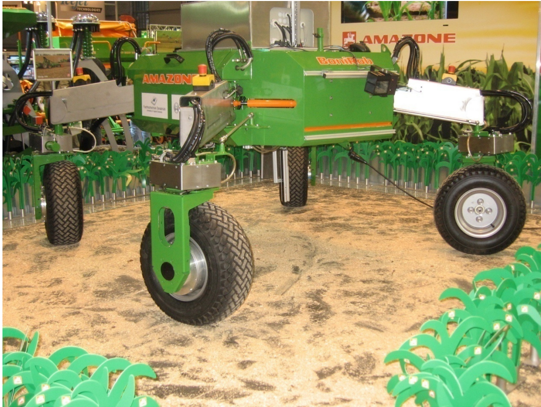
Fig .5 'Bonirob' autonomous crop plot inspection and monitoring vehicle.
