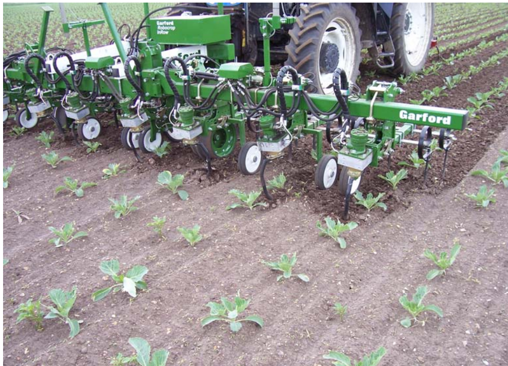
The Robocrop in row – hoes weed around each individual plant
