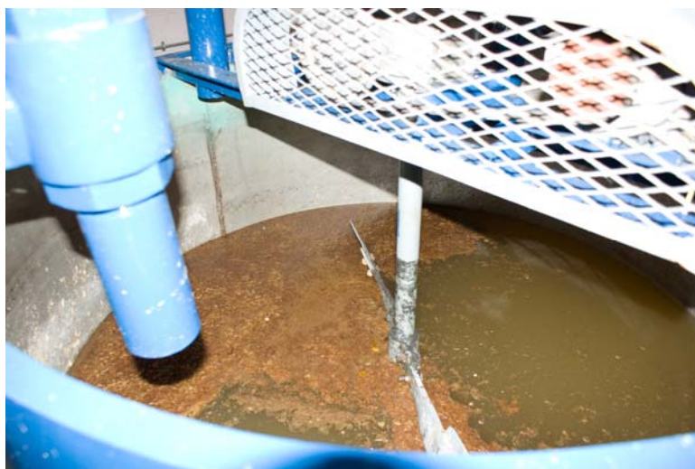
The pulping drum – making adjustments to this process was key in improving the technical performance of the pulp
