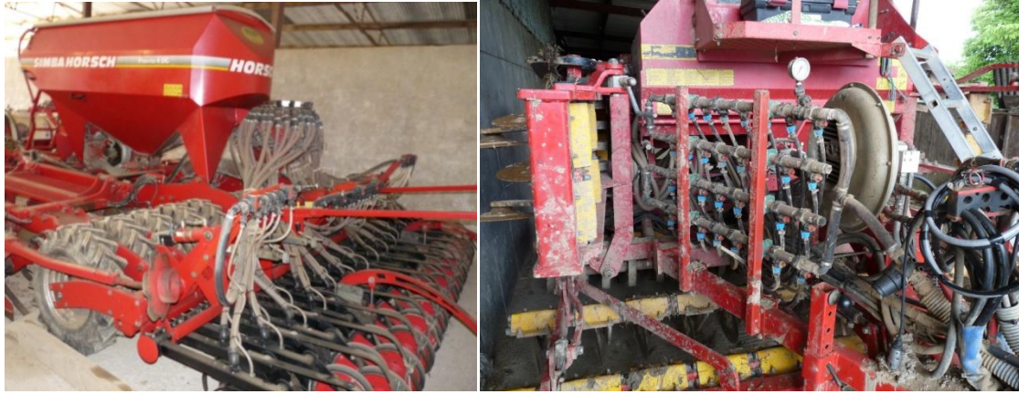
Figure 6, Some of the liquid application equipment used in Ireland to “row load” nutrients at planting
