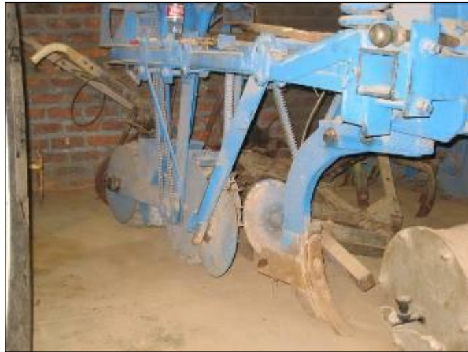
Figure 18. Native rangeland grass sowing equipment Worcester Natural Veld Research station South Africa
