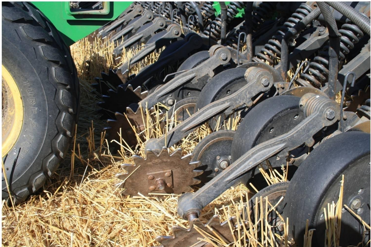
Zero Till disc seeder, showing the residue handling capabilities
